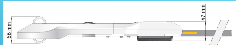
Figure 2.1 The dimensions of the CNR 4 with CNF 4 ventilation unit, side view
