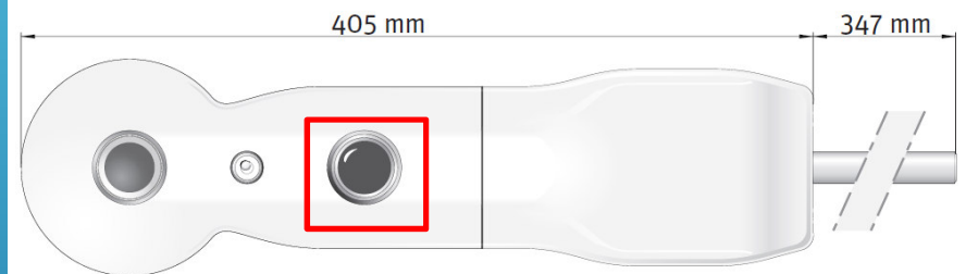
Figure 2.2 The dimensions of the CNR 4 with CNF 4 ventilation unit, top view
