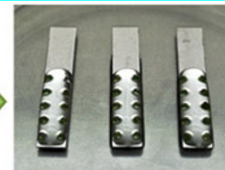
Hardening of the gel by CaCl 2 sol.
