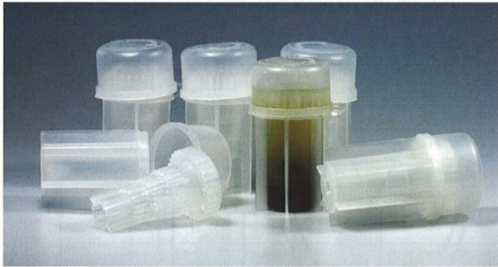
Fig. example of commercial flotation kit; simple plastic single use vials are used for zinc sulphate flotation without the centrifugation.
