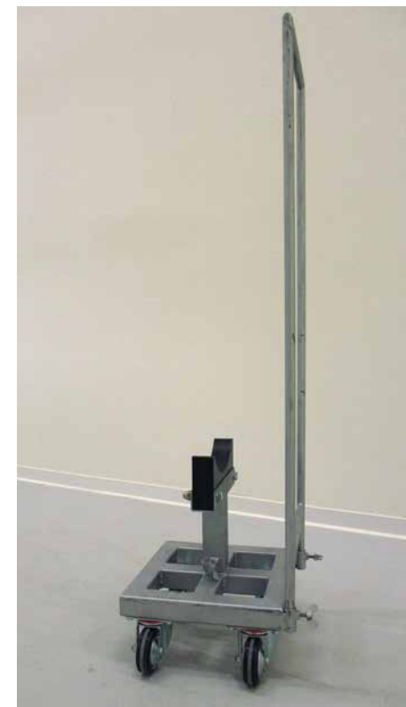
Fig. 16: Dolly with half-shells for handling the tapestries rolled-up onto folded spiral-seam pipes.
