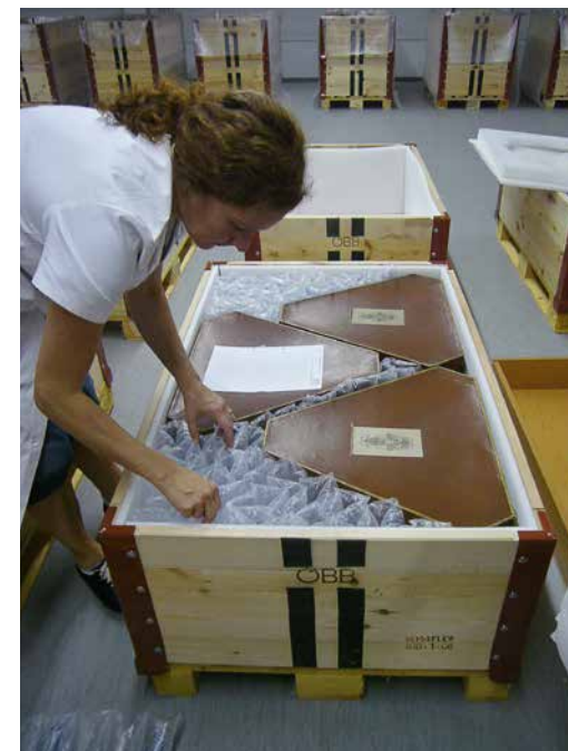
Fig. 17: ÖBB stacking frames fitted with Ethafoam, for the relocation of costume-accessories. Padding of any existing voids with LDPE-air cushions.
