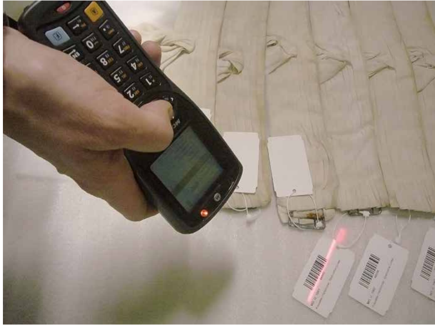
Fig. 4: Scanning a barcode with the laser scanner (Motorola MC 1000 Scanner) for location logging in TMS.
