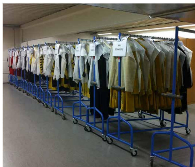
Fig. 15: Mobile clothes racks with Z-shaped base frames can be nested into one another to save space.
