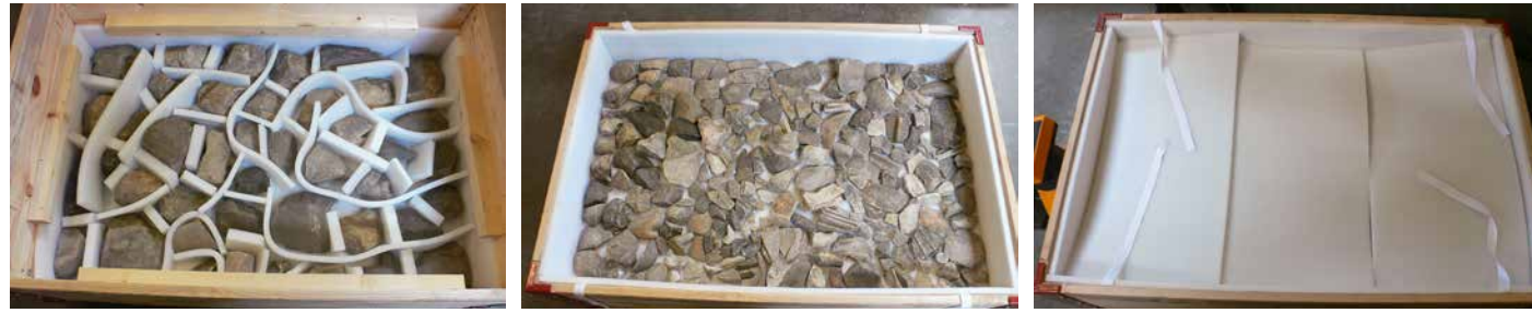
Fig. 74 a First and second layer of packed fragments with enclosing Ethafoam cover.
