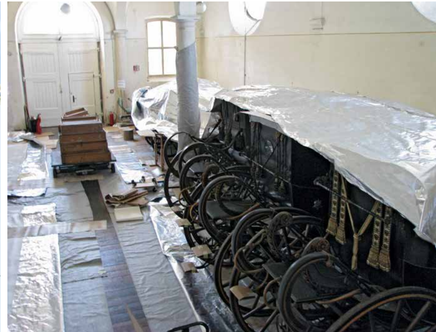
Fig. 5: Nitrogen tent for anoxic nitrogen treatment of the carriages from the Imperial Carriage Museum.
