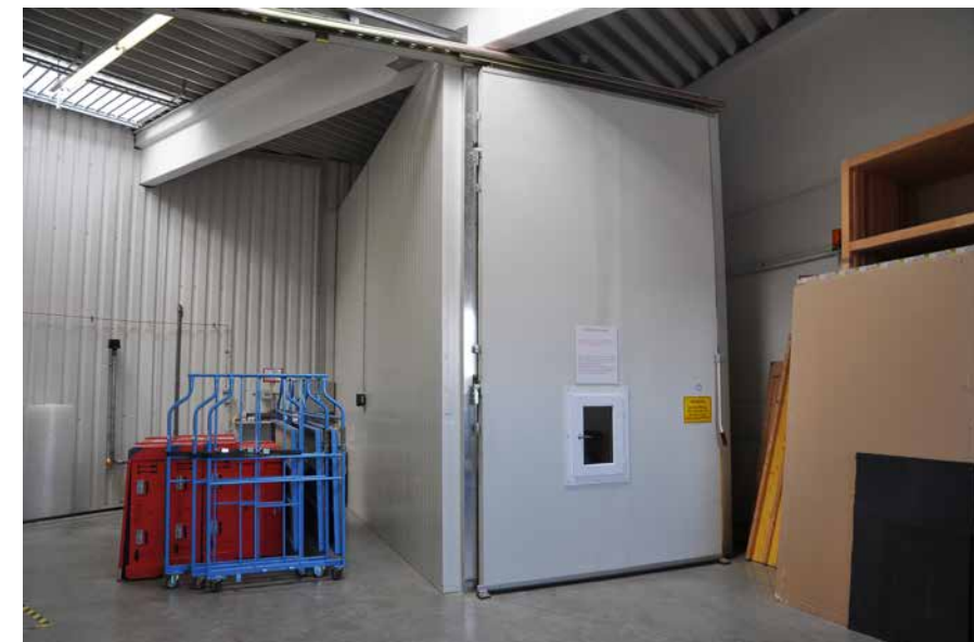
Fig. 1: First anoxic nitrogen treatment chamber in the KHM, which was continually in use from 1998 until 2011.
