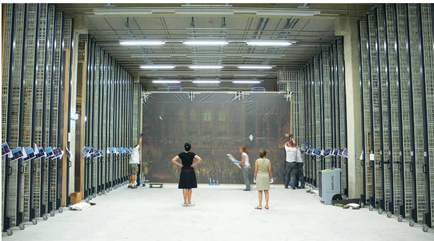
Fig. 1 b: At the new centralised storage facility, there is room even for the largest formats on the wire mesh walls of the pull-out picture racks. Picture of a large format wrapped in PE foil, taken during the relocation campaign.
