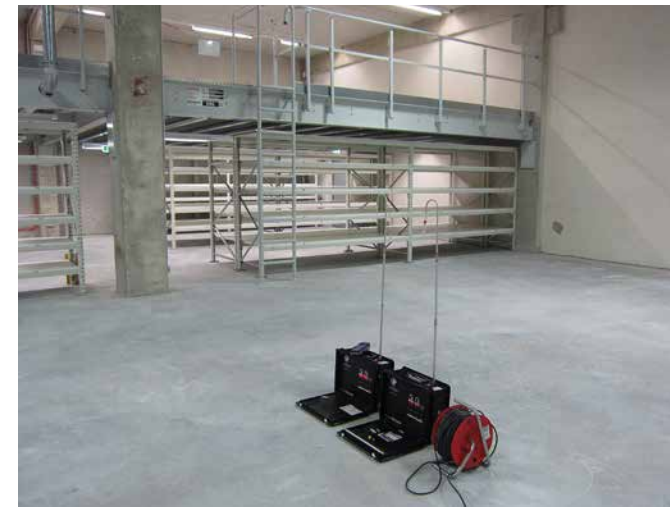
Fig. 1: First air pollutant measurement carried out by IBO Innenraumanalytik OG in August 2011; view of the storage area on F1, Imperial Carriage Museum/Court Wardrobe with mezzanine (intermediary steel platform) during indoor air sampling.
