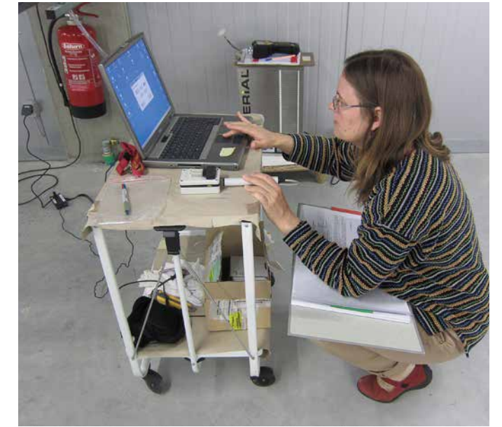
Fig. 11 b: Collecting the corrosion data from the bronze sensor, which was in place as shown in fig. 11 a for 21 days.
