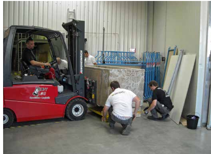
Fig. 81: Transfer of the sarcophagus with forklifts onto a transport pallet made of formboards and wooden beams.
