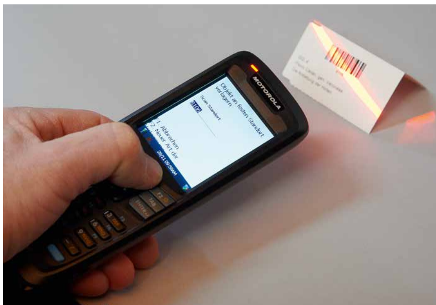
Fig. 5: A barcode label is scanned for the software “BarApp” with a laser scanner.
