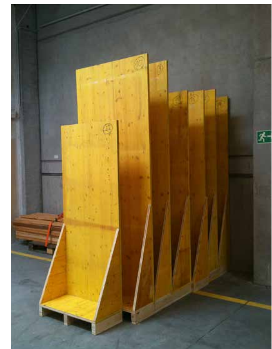
Fig. 38: L-shaped wooden boards for the transport and storage of stone reliefs and tombstones from the Collection of Greek and Roman Antiquities.
