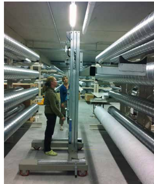
Fig. 64: Custom-made mechanical, mobile lifting apparatus (Stefan Fleck/Bernard Rendl GmbH) for manipulation of the commercially available folded spiral-seam pipes made of galvanised steel sheeting for later storage of the Kunstammer tapestries.
