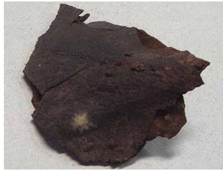
Fig. 39: Leather fragment from a shoe – light, furry mould spots on the exterior.
