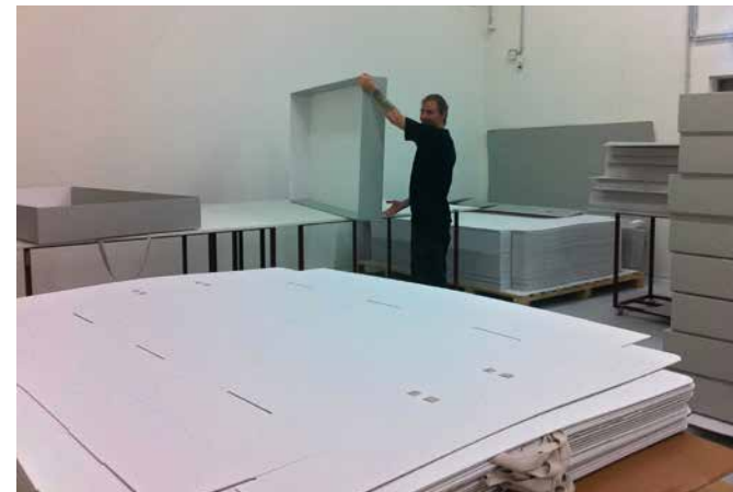
Fig. 33 a Acid-free cardboard boxes by the Klug-Conservation company for the storage of oversized textiles. On the left, during assembly by an employee of the Japico company. On the right, with stored regalia of the English Order of the Garter.
