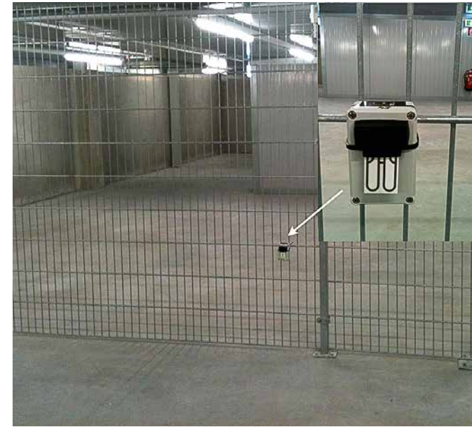
Fig. 11 a: Use of the AIRCORR I logger with a bronze sensor in the still empty F2, Coin Collection, climate box.
