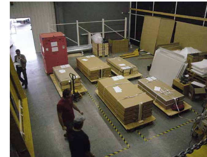
Fig. 12: Storage facility Inzersdorf, pre-placement of the packed objects for transport by the art moving company. The demarcations on the floor indicate the size of the truck.
