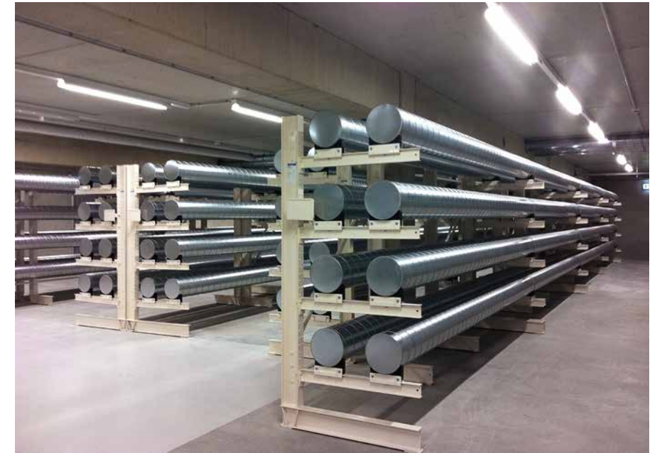
Fig. 11: Shelves for storage of the tapestries rolled onto folded spiral-seam pipes.
