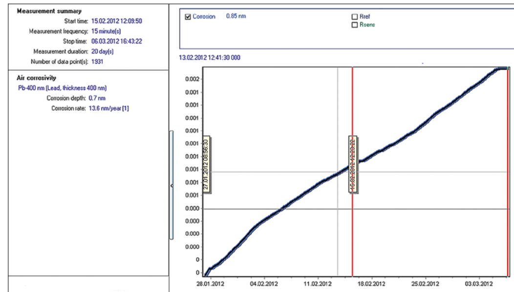
Fig. 10: Results of the evaluation of the lead sensor placed in F3, Imperial Carriage Museum/Court Wardrobe, gained by using the associated software. Like with all sensors in the MUSECORR system, the lead sensor can also be used more than once in different locations for testing the corrosive potential of the surrounding atmosphere. In the evaluation shown here, the measurement period in F3, Imperial Carriage Museum/Court Wardrobe is delimited by the two red lines (from February 15 th , 2012 to March 6 th , 2012). The evaluation of this section of the corrosion curve shows a corrosion depth of 0.7 nm and a corrosion rate of 13.6 nm per year. According to the project leaders at MUSECORR, this corresponds to a potentially non-corrosive environment for objects.
