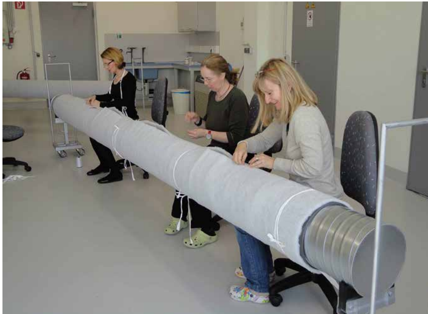
Fig. 8: Wrapping of the folded spiral-seam pipes with polyester fleece (third step).
