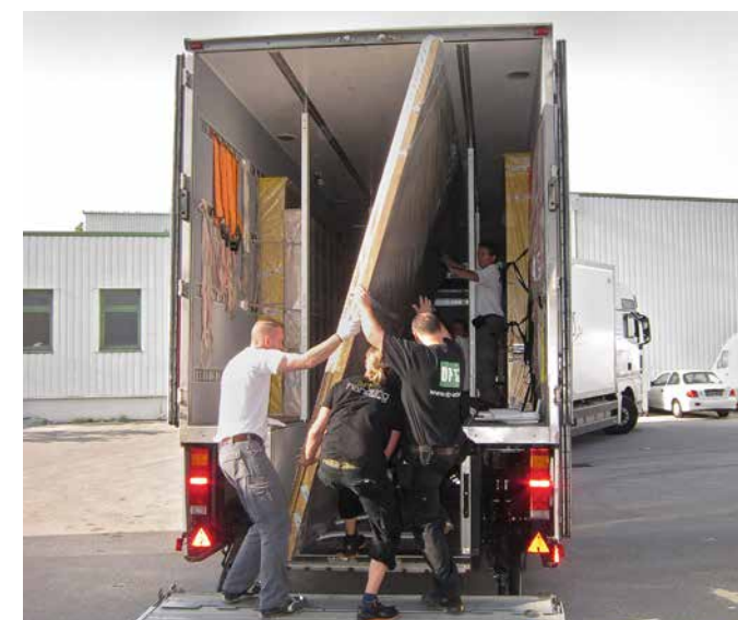
Fig. 41: This special tandem trailer from the Kunsttrans company has a maximum diagonal of 386 cm, due to a lowered loading space inserted between the wheel base.
