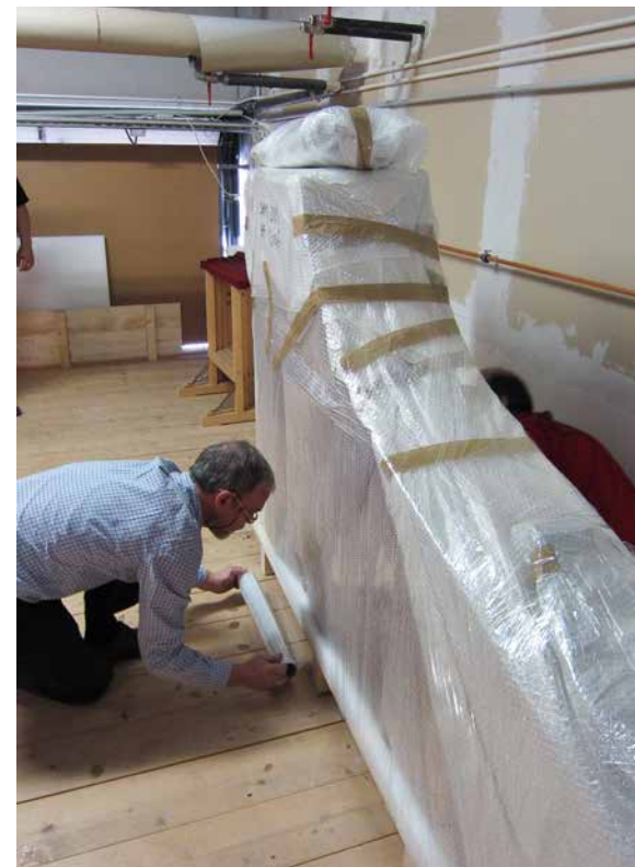
Fig. 6: The encased piano and its transport board are wrapped together in PE sheeting.
