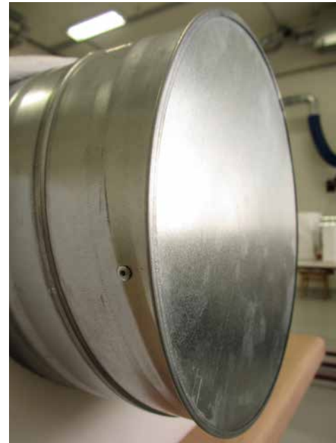
Fig. 9: Riveted lids of the folded spiral-seam pipes.
