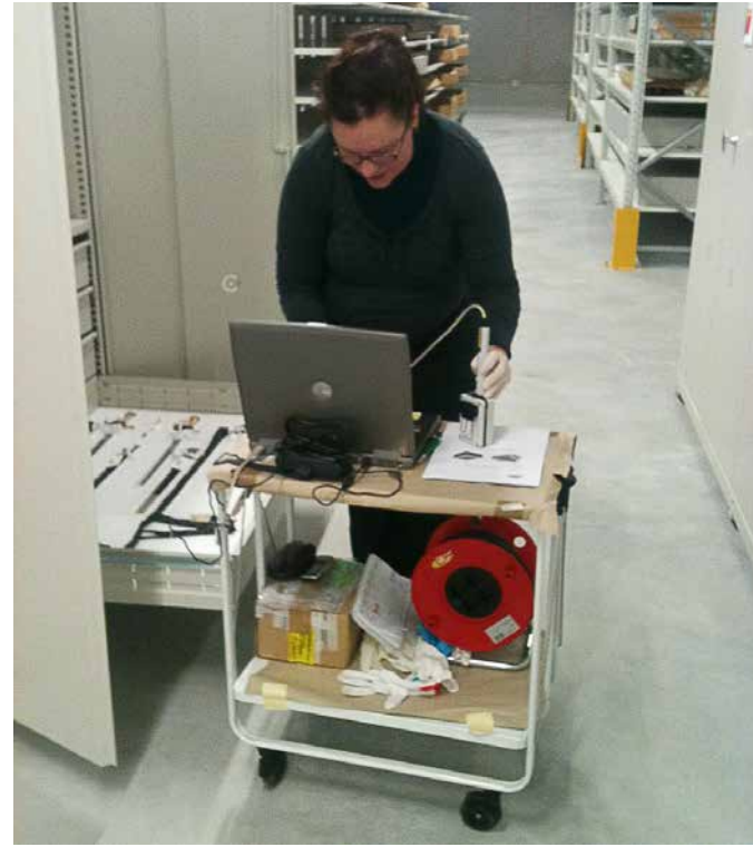
Fig. 9 b: Collecting the corrosion data from the lead sensor, which was in place as shown in fig. 9 a for 20 days.
