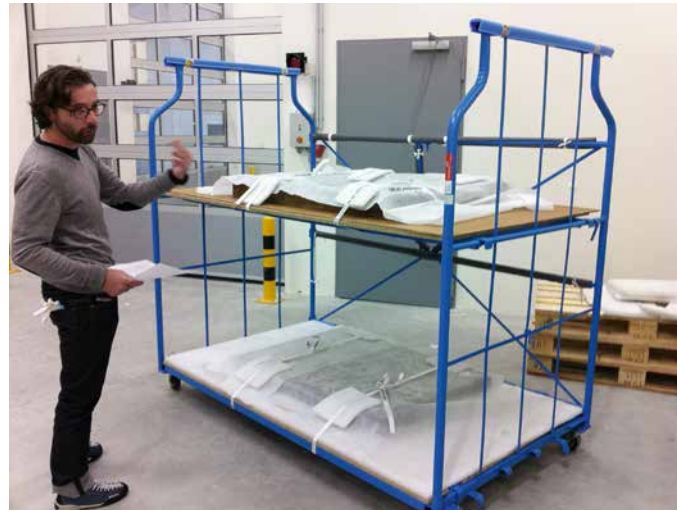
Fig. 31: Corlette storage rack with insertable shelves for the transport of stone panels from the Kunstkammer.
