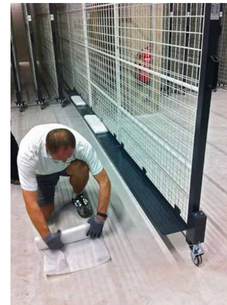
Fig. 62: Attachable support element for large-format or heavy paintings.
