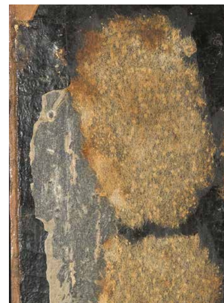
Fig. 14: Several types of paper were used as facing materials over the years. Some of the facings with Japanese tissue paper are noticeably discoloured. Analysis of the binding medium of these protective papers, which had only been applied in the 1980s, has revealed that the browning and crystallisation phenomena stem from the use of honey in the consolidating material.
