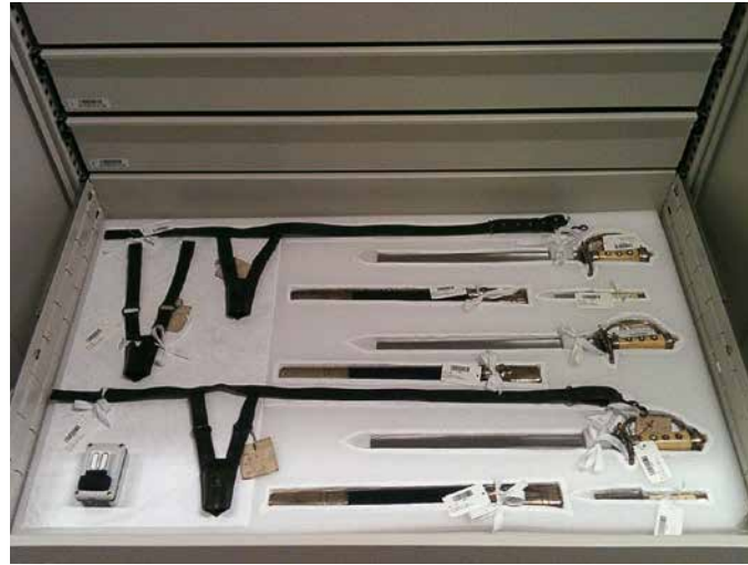
Fig. 9 a: Use of the AIRCORR I logger with lead sensor (below, left) in a drawer already filled with artefacts in F3, Imperial Carriage Museum/ Court Wardrobe.
