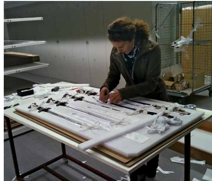
Fig. 20: Preparation of custom-fit blocks of Ethafoam, carved to the shape of the object and lined with Tyvek, for securing the objects within the drawers.
