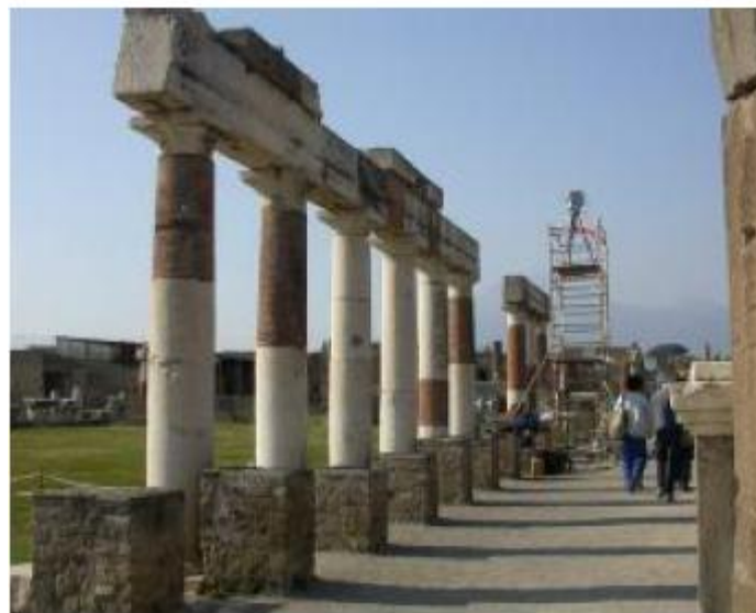
Fig. 2: The scanner 3D has been placed at a high position to avoid the shade areas due to the presence of people. It surveys a 360° angle area.
