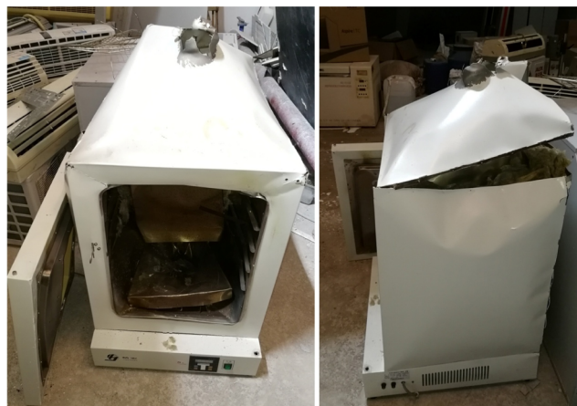
Figure 1. Front and side views of the oven after explosion of the hydrothermal reactor.
