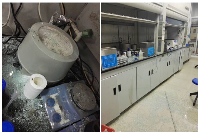
Figure 2. Fume hood damaged by explosion of perchloric acid–organic compounds digestion reaction. (Reproduced with permission from Professor Qin Kuang.)
