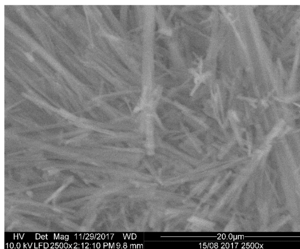
Figure 11. (left) Results of seeded cooling crystallization of IMC from ethanol at 5 °C and high supersaturation. (right) SEM image of crystals obtained with a seed loading of 1%.
