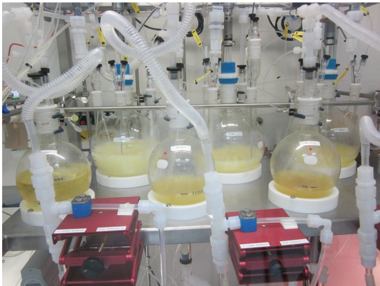
Figure S28. Photograph of extraction system running.
