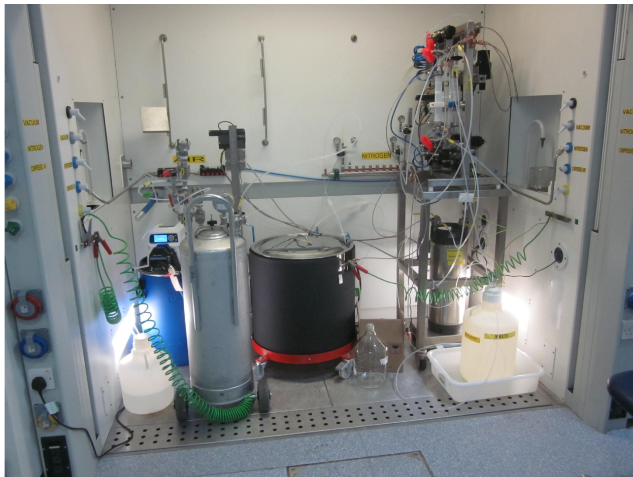
Figure S33. Fume hood containing water bath and S_NAr reactor with automated HPLC dilution cart.
