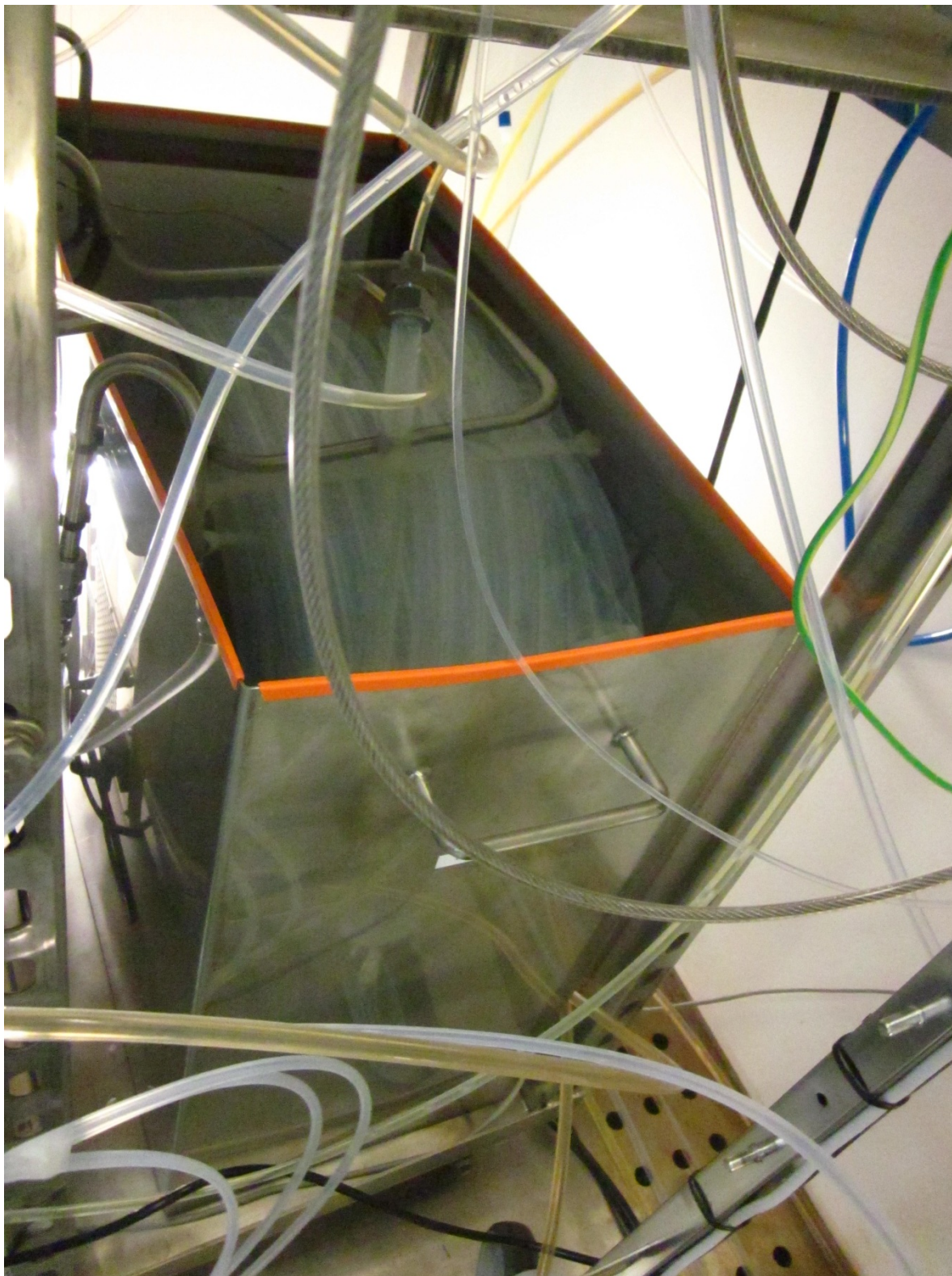
Figure S38. Photograph of deprotection gas/liquid PFR in thermostatic bath.
