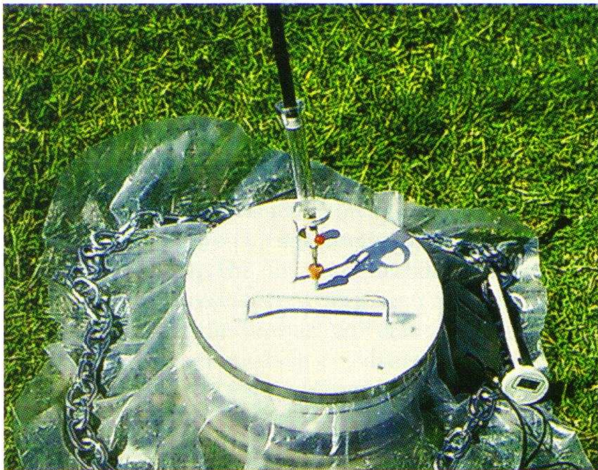
FIGURE 11.14 A field chamber that allows measurement of respiration gases. (From Pollution Science , 1996, Academic Press, San Diego, CA.)
