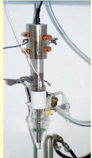
Ti alloy horn, minimum lenght is a half-wavelength of sound in a material, 26 cm for 20 kHz in Ti, multiples of 13 cm
