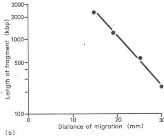
Agarose gel electrophoresis of DNA. (a) Separation of: 1, different forms of DNA of plasmid pBR322; 2, fragments of DNA (lengths indicated in kbp) derived from plasmid pBR322 by double-digestion with restriction endonuclease *Bam* HI and *Bgl* I; (b) Plot of length of DNA fragment (log scale) against distance of migration (linear scale) of data from (a) 2, illustrating linear relationship.
