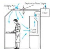
ULPA/All Totally contained laboratory work area Hazardous waste analysis, toxicology, chemical and acid fume ventilations, safety stations, explosion proof and flammable storage
