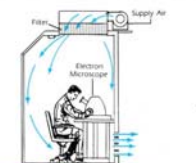
Isolation Room Dust/draft free, temperature controlled modules Microscopy, clinical chemistry, forensic chemistry, spectroscopy and chromatography.
