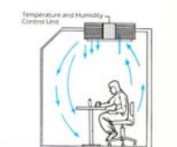
Environmental Room (Temperature and humidity controlled environment) Computer applications, pathology, microbiology, material storage, ASTM testing
