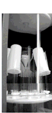
Figure 2. Twenty-position component rack with PTFE-based glass rods.
