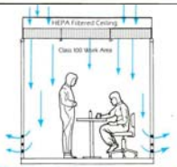
Micro-Electronic Assembly Continuous clean room systems Quality control and testing, electronic packaging, robotics, and static protection, HEPA filtered positive pressure work area
