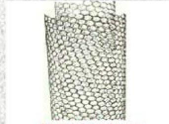
A multi-shell nanotube image (Ebbesen, T. W., 1994. Annu. Rev. Mater. Sci. 24:235-64. courtesy of NEC/Handa)
