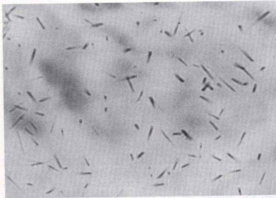
FIGURE 2.10 Each fission track (about 16\ \mu\text{m} in length) in this apatite crystal is the result of the radioactive decay of a uranium atom. The crystal, which has been etched with hydrofluoric acid to make the fission tracks visible, comes from one of the dikes at Shiprock, New Mexico, and has a calculated age of 27 million years.
