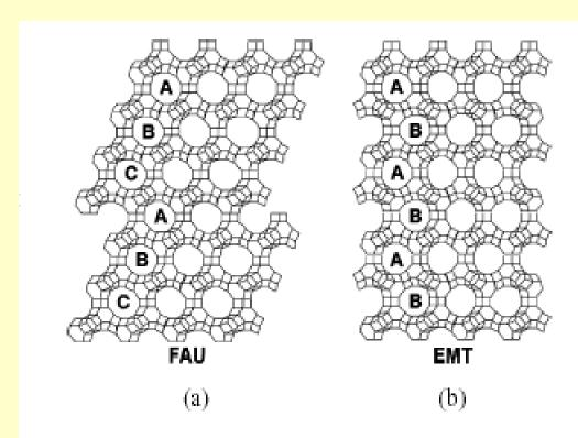
Fig. 1. Structure of zeolite Y: (a) cubic polymorph known as FAU with ABCABC... stacking, (b) hexagonal polymorph known as EMT with ABABAB... stacking.
