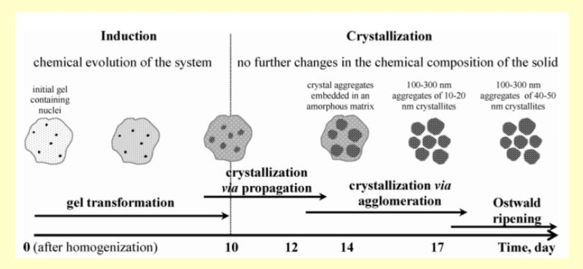
crystallization mechanism of FAU-type zeolite under ambient conditions
