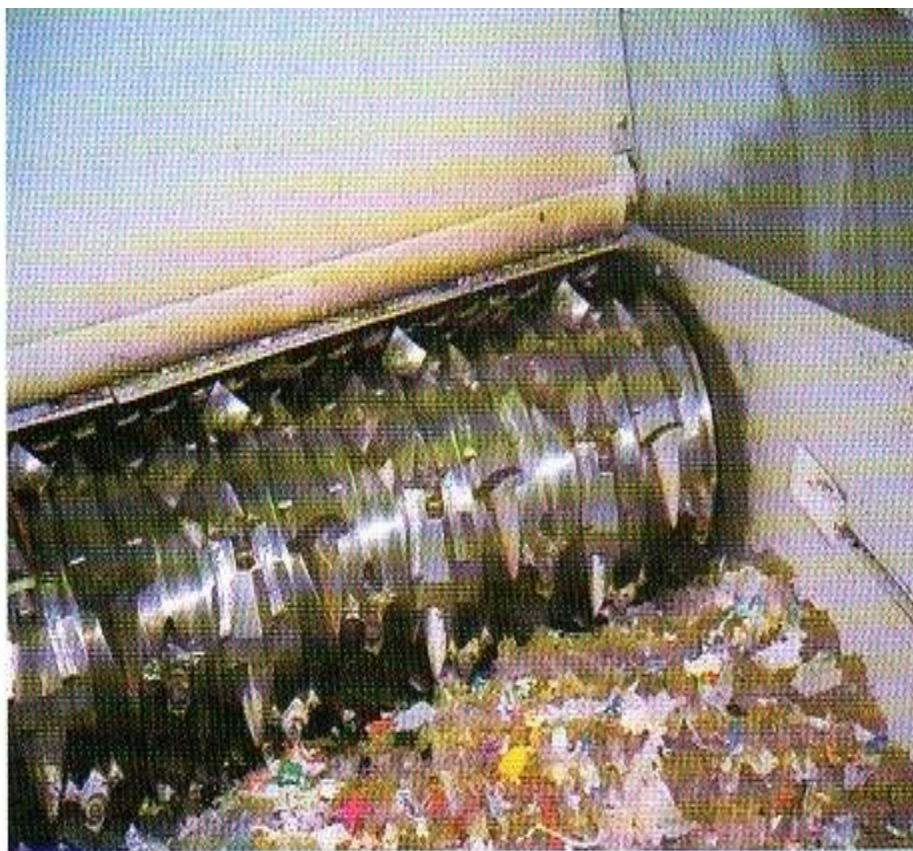
Mixed plastic input is preshredded to reduce it to particle sizes of 10 to 40 mm.
