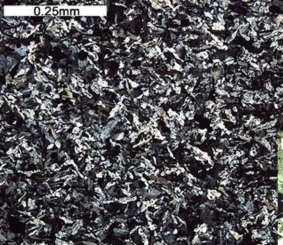
Subophitic albite-carbonate rock, altered mafic lava or dolerite. Meurastuksenaho, Kuusamo Schist Belt. Crossed polarisers. Photo Erkki Vanhanen.
