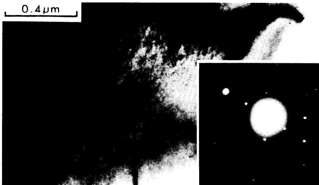
Fig. 27. Bright-field image and corresponding diffraction pattern from Pu-substituted zirconolite after 4 days storage near room temperature. The diffuse rings in the diffraction pattern are from the carbon substrate (Clinard et al. , 1984).
