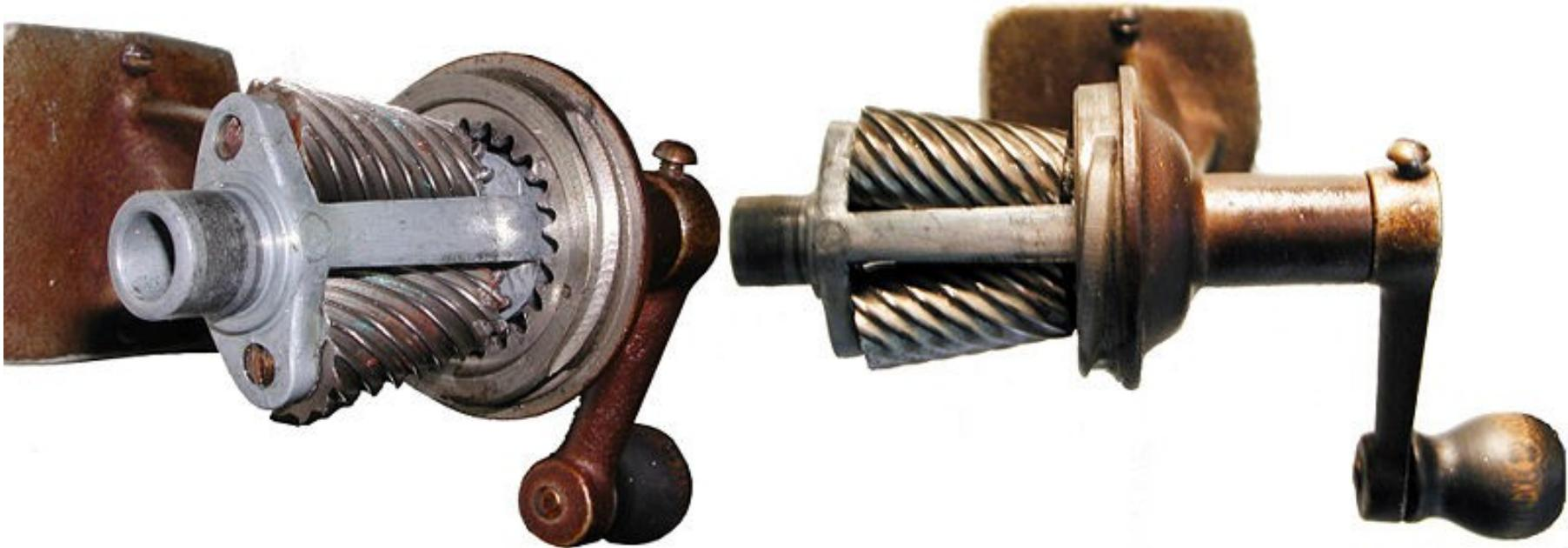
The mechanism of a pencil sharpener with stationary annulus and rotating planet carrier as input. Planet gears are extended into cylindric cutters, rotating around the pencil that is placed on the sun axis. The axis of planetary gears join at pencil sharpening angle.
