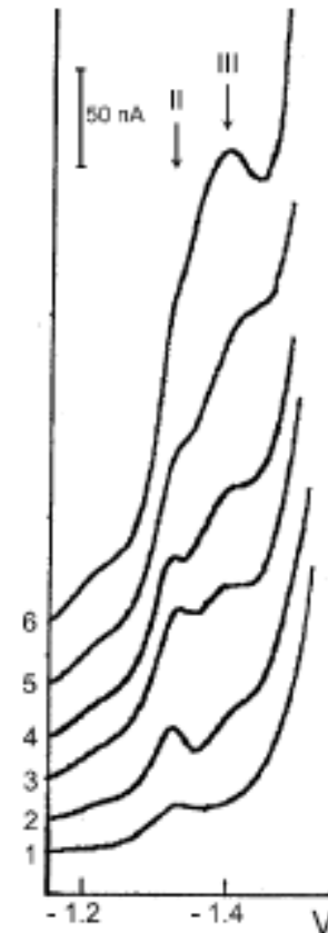
Fig. 7 Differential pulse polarographic analysis of CT-DNA modified by ORGANObisPt. DNA at a concentration of 0.4 mg/mL in 0.3 M ammonium formate with 0.01 M phosphate buffer, pH 6.8. Curve 1 : control, unmodified DNA; curves 2-6 : DNA modified by ORGANObisPt at r_b = 0.001, 0.003, 0.005, 0.007, 0.01 , respectively; the arrows marked II and III indicate potentials E (against saturated calomel electrode) at which native or denatured DNA samples yielded DPP peaks II or III, respectively (see text)
