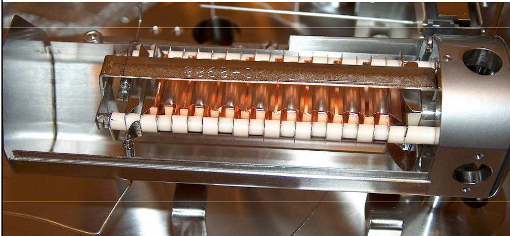
Discrete-dynode electron multiplier
