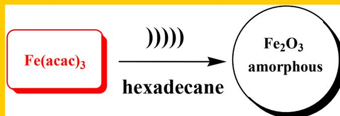
**Amorphous product, by heating to 700 °C converted to  $\alpha$ -Fe<sub>2</sub>O<sub>3</sub> 20–40 nm**
