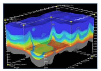
much more accurate in 3D, as property distributions can be taken into account more accurately and all lateral effects can be taken into account. The image shows modeled overpressure distributions in a Gulf of Mexico model.
