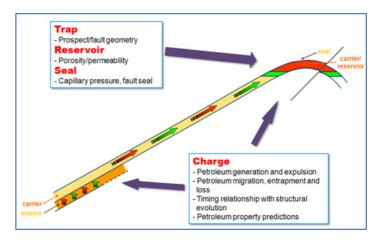
evolution of the trap and its properties. The same geological principles apply in both conventionals and unconventionals: in conventionals, exploration is directed at the expelled and migrated hydrocarbons, while in unconventionals the retained hydrocarbons are of interest.
