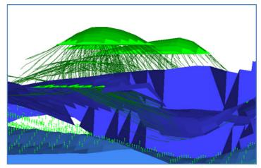
which represent potential reservoirs. The image shows detail from a 3D model with the vectors indicating petroleum expulsion from source rocks modeled with Darcy flow, and the dark green Flowpath flowlines indicating petroleum migration in higher-permeability units into petroleum accumulations. The dark blue colours show salt.
