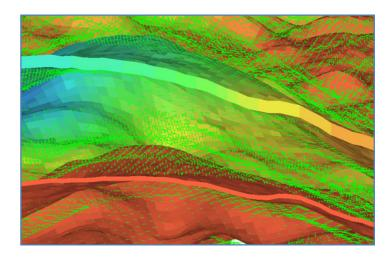
determined. Depending on the geological conditions such as rapid recent generation and migration, these can be important. They are essential for slow oil migration processes in shale resource plays. The image shows Darcy flow (vectors) of full 3D pressure controlled upward and downward expulsion from two source layers in the pre-salt in Brazil.
