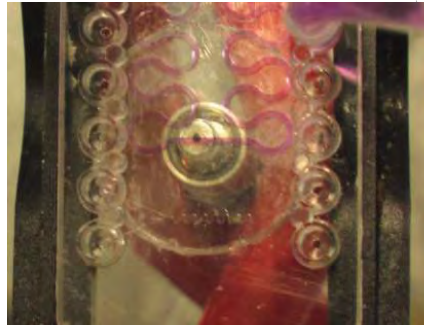
600 µm optical fibre aside of 640 µm wide channel
