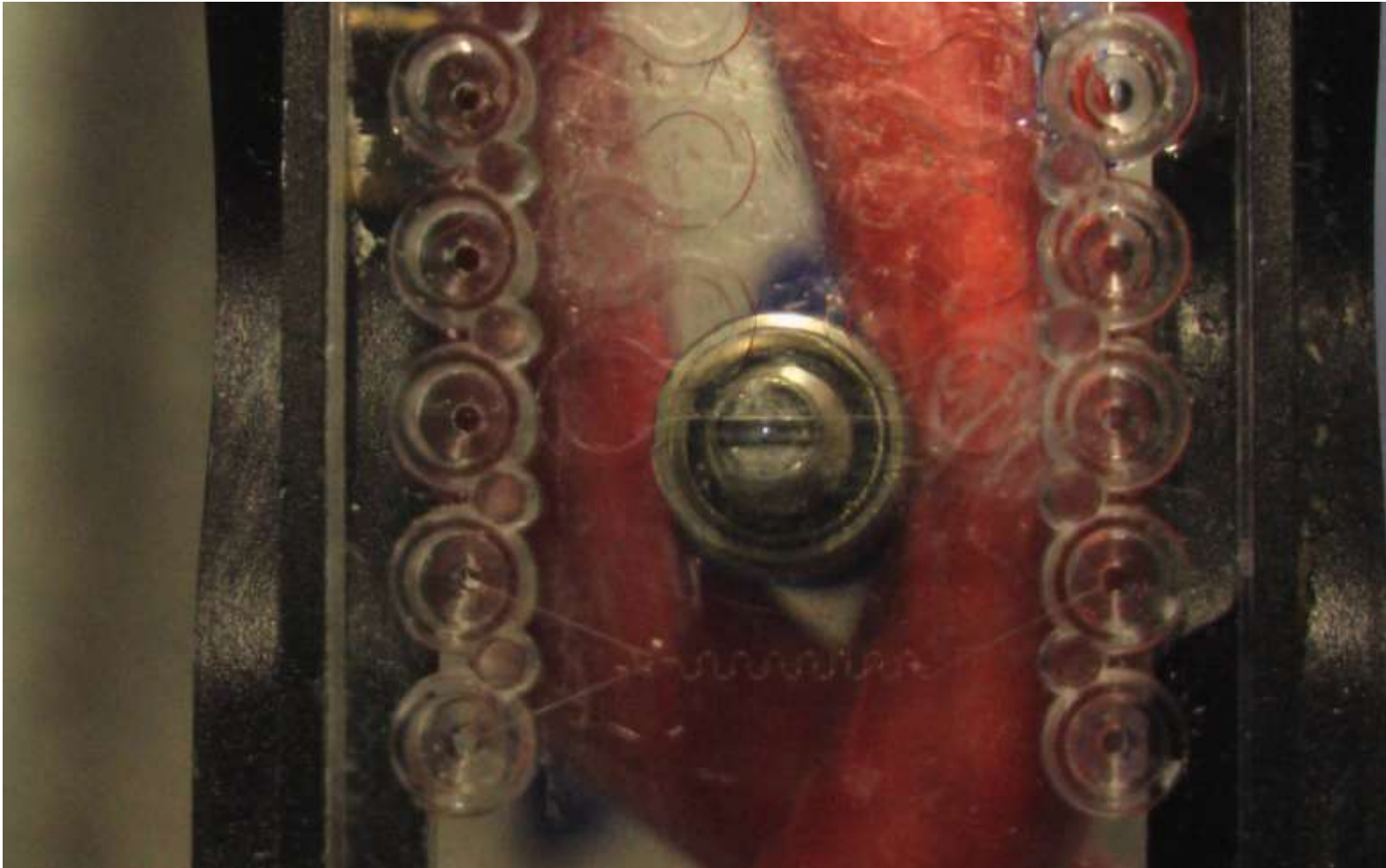
100 µm optic fibre in the centre of 640 µm channel
