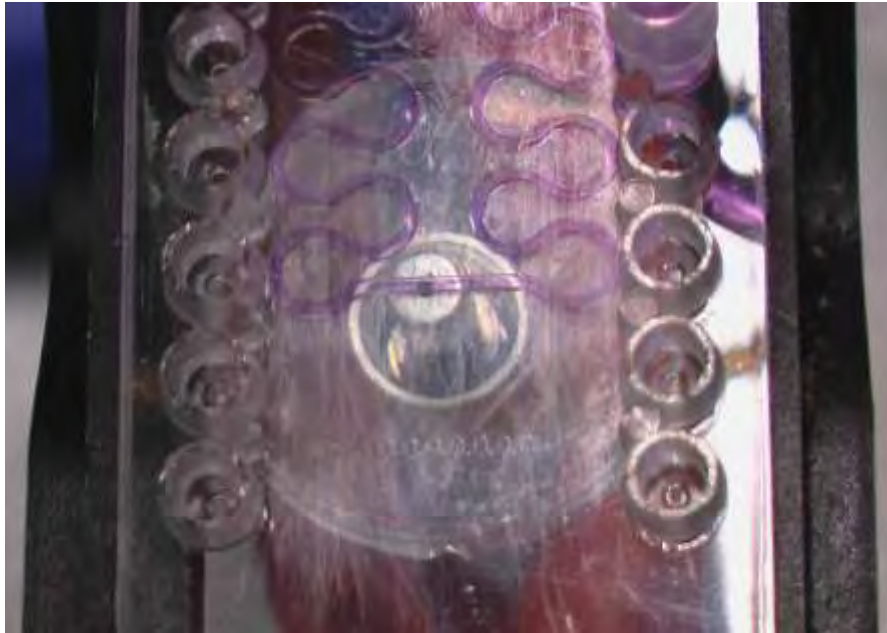
600 µm optic fibre across the 640 µm wide channel
