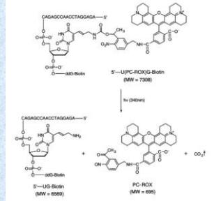
Fig. 2. DNA product 5'-UPC-ROXG-Biotin, formed by incorporating a dUTP-PC-ROX into a primer in a polymerase reaction and its photocleavage, producing DNA Fragment 5'-UG-Biotin and PC-ROX. MW = molecular weight.
