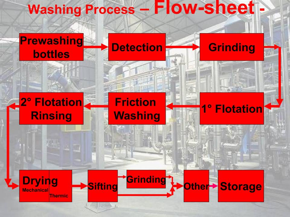
The Bottles and Flakes Washing is performed by following combined actions: mechanical (friction), chemical (chemical product), physical (high temperature)
