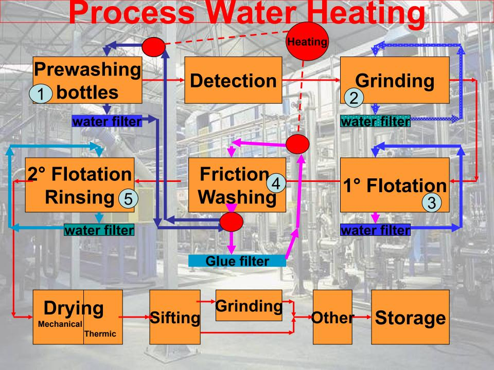
In every Washing Step Water is continuously conditioned with ecological Chemicals Products for the perfect elimination of Pollutants and Glue
