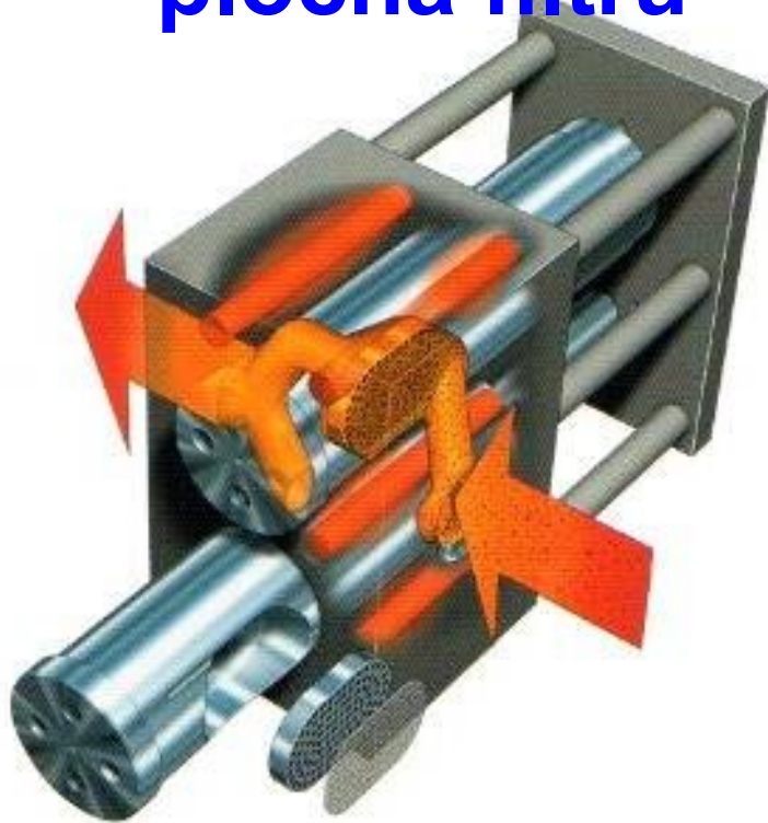
3D model of a continuous screen changer type LK-SWE in screen change position
