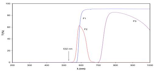
Figure 5a. Transmission spectra of selected optical filters
