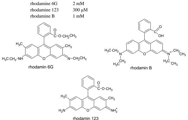
Figure 6: Structure of the rhodamine dyes
