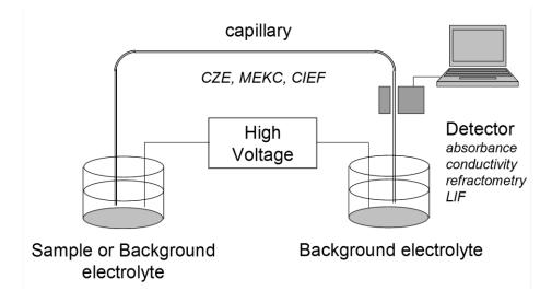
Figure 2. Scheme of the instrumental setup of capillary electrophoresis
