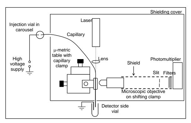
Figure 3. Scheme of CELIF instrumentation.
