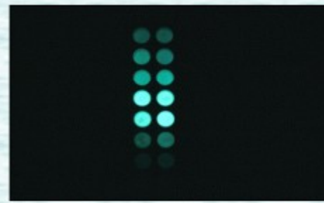
Luminescent response to a dilution series of a genotoxicant on a microtiter plate, photographed only by the light emitted by the bacteria
