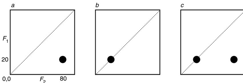
Suppose that in some unspecified two-dimensional spectrum a peak appears at  $F_1 = 20$  Hz,  $F_2 = 80$  Hz (spectrum *a* above). The interpretation of this peak is that a signal was present during  $t_1$  which evolved with a frequency of 20 Hz. During the mixing time this *same* signal was transferred in some way to another signal which evolved at 80 Hz during  $t_2$ .
