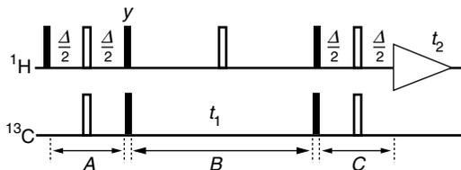
The pulse sequence for HSQC. Filled rectangles represent  $90^\circ$  pulses and open rectangles represent  $180^\circ$  pulses. The delay  $\Delta$  is set to  $1/(2J_{12})$ ; all pulses have phase  $x$  unless otherwise indicated.
