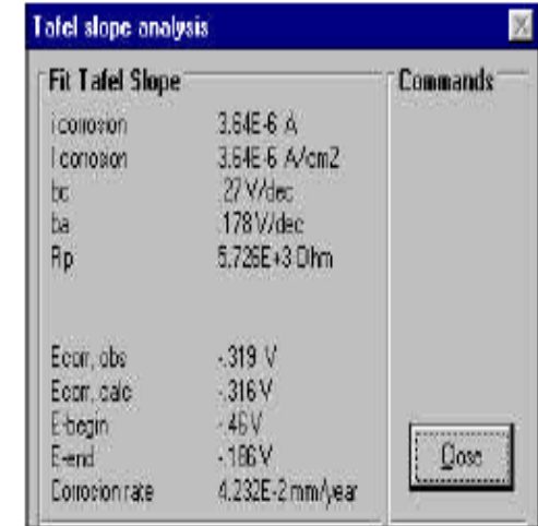
Figure 5: GPES window for showing the results of Tafel analysis.
