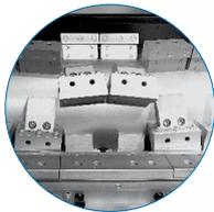
Blades made of high-strength, hardened and tempered special steel
