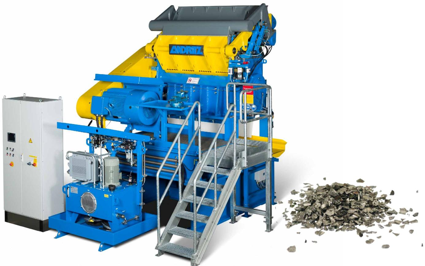
**The newly designed UG Granulator series from ANDRITZ MeWa processes large-scale waste products, producing results sorted by type of material.**
