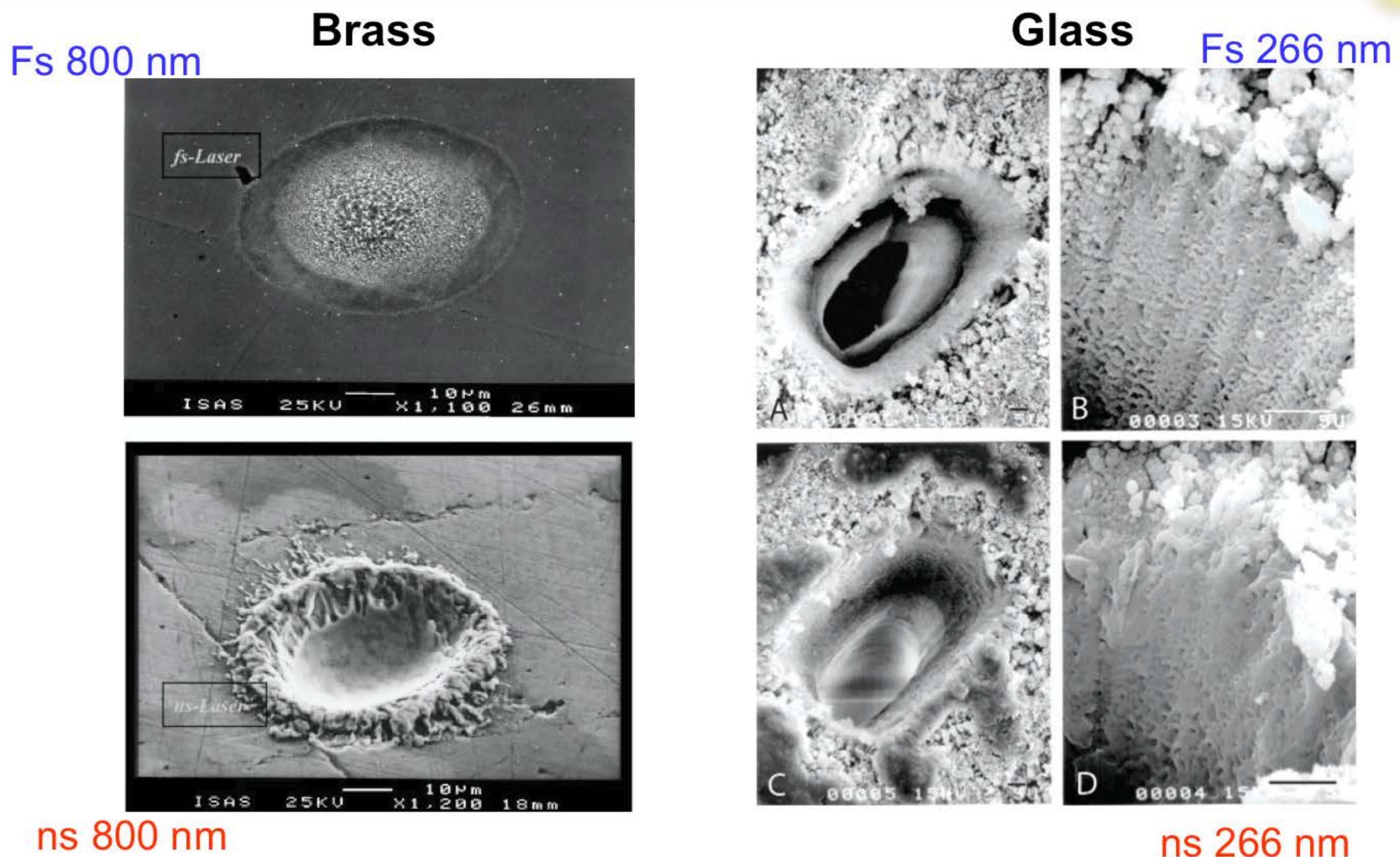
**FIGURE 4.** Fs- and ns-ablation of polished brass directly revealed different ablation mechanism. In both cases no beam shaping was used. Whereas the fs crater has a clean rim, the ns crater shows the typical pattern of melting. (Modified from Elsevier, Spectrochim. Acta B 55(2000)1771).
