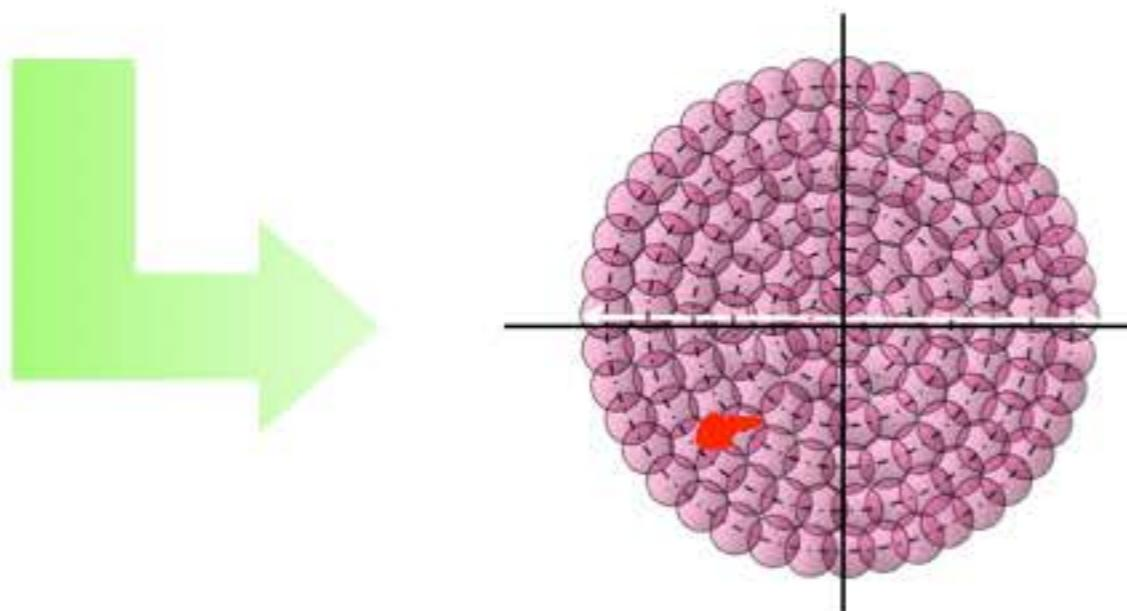
*Crater of  $40\ \mu\text{m}$  diameter to make sure to ablate the particles of interest*
