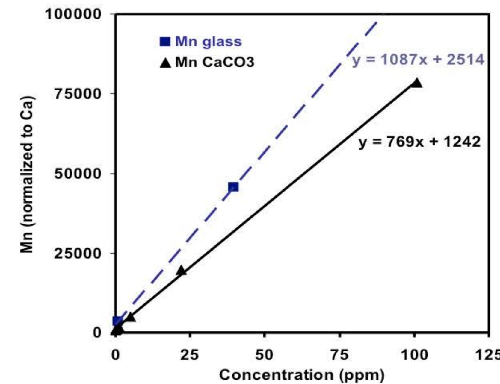
Fig B Calibration with certified glasses and  $\text{CaCO}_3$  standards. ns 266 nm laser
