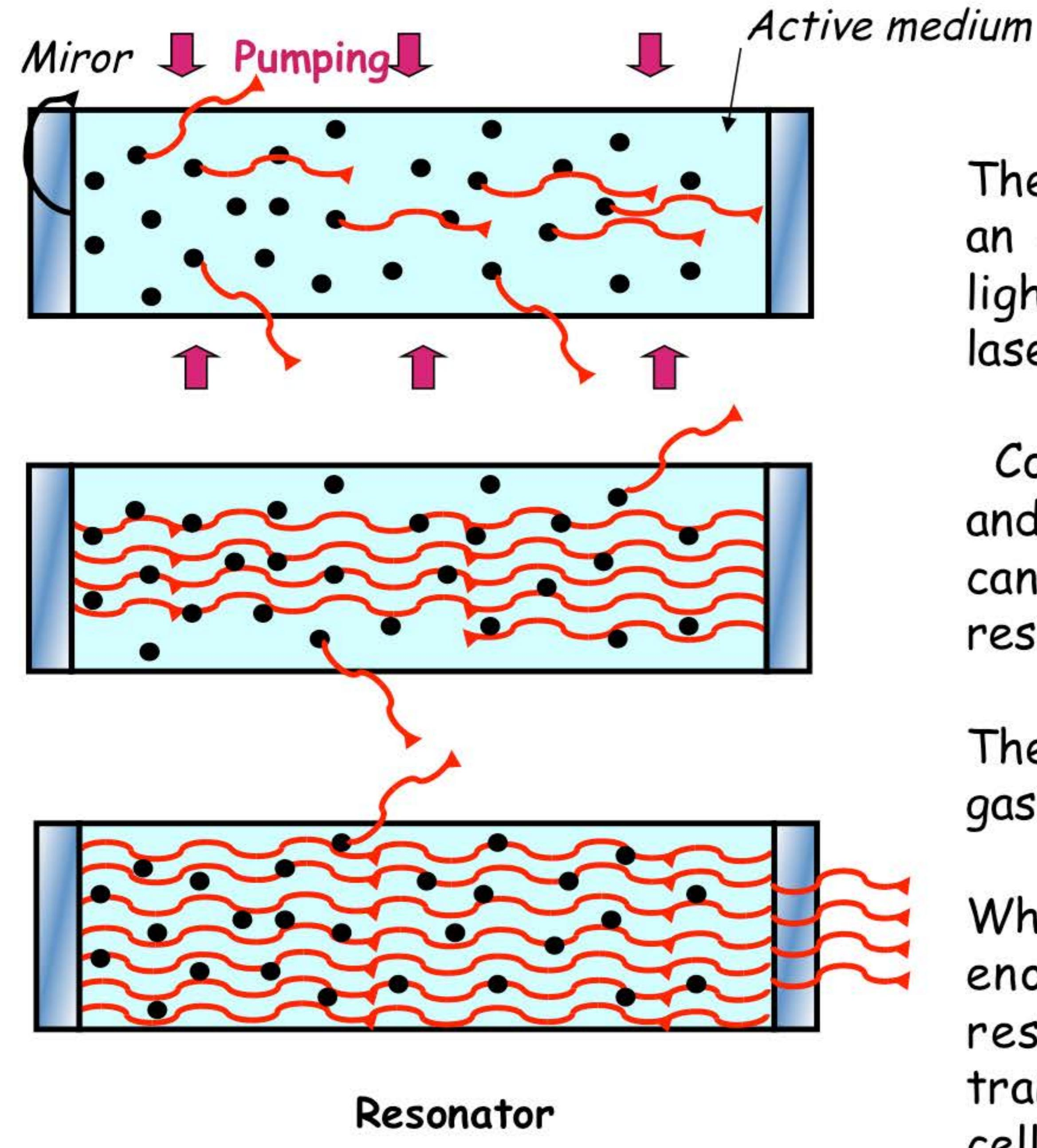
The population inversion is triggered by an external source of energy (pumping: light flash, electric source, or even lasers)
