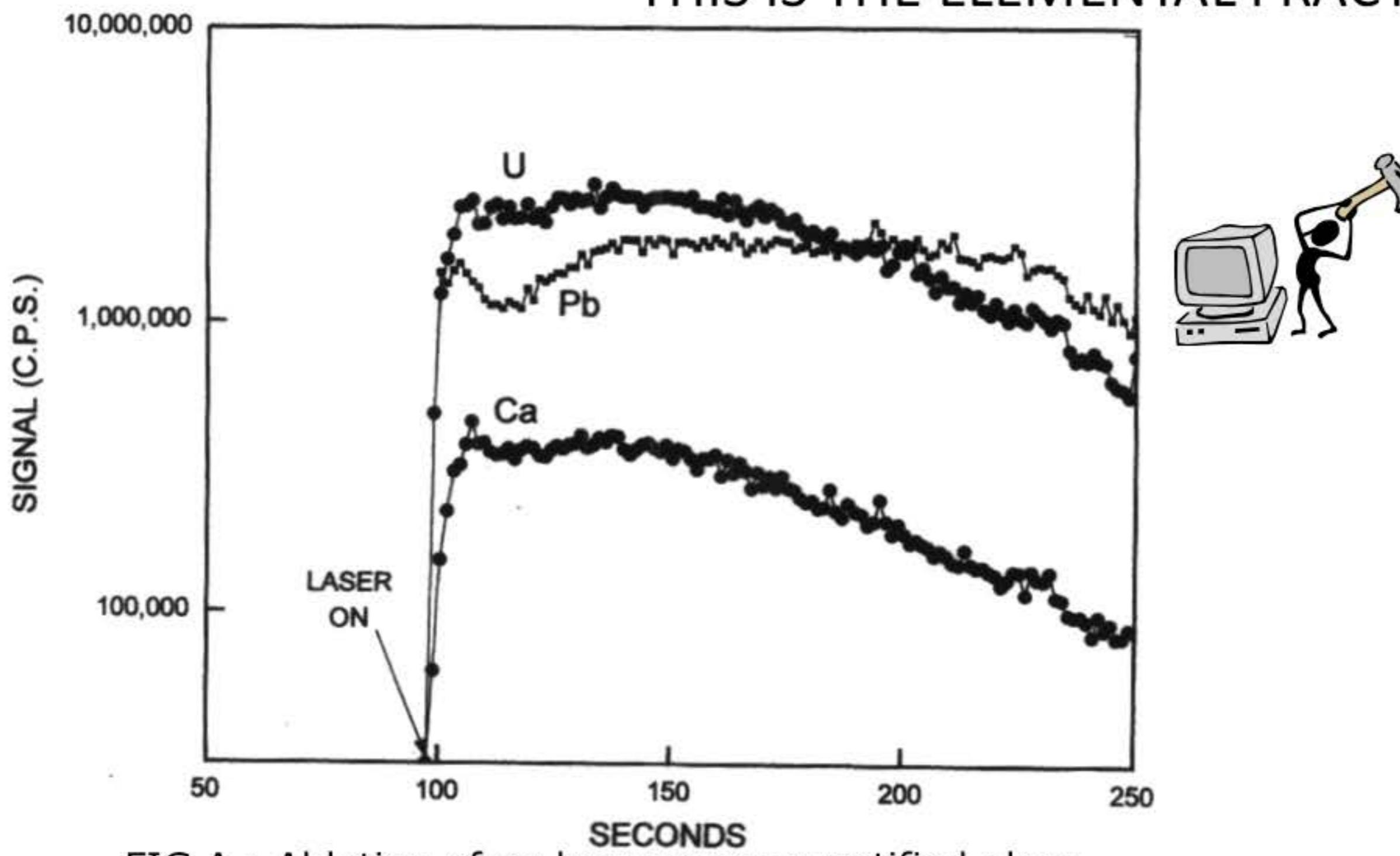
FIG A : Ablation of an homogenous certified glass sample (NIST 610). ns 266 nm laser
