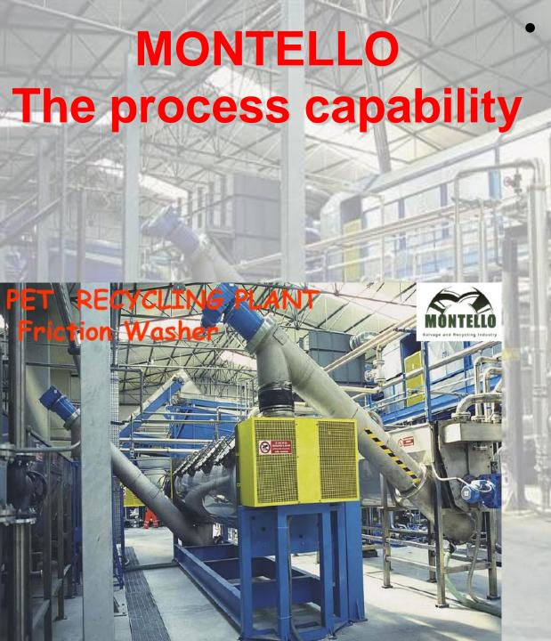
The PET recovery plant has a process capability up to 20.000 ton/year of PET post consumer bottles with a potentiality of 3.600 kg/hour input and 3.000 kg/hour output.
