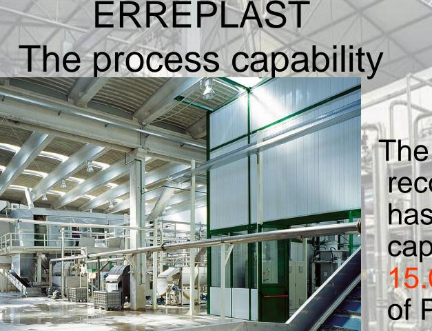
The plastic recovery plant has a process capability up to 15.000 ton/year of PET post consumer bottles with a potentiality of 2.500 kg/hour input and 2.000 kg/hour output.
