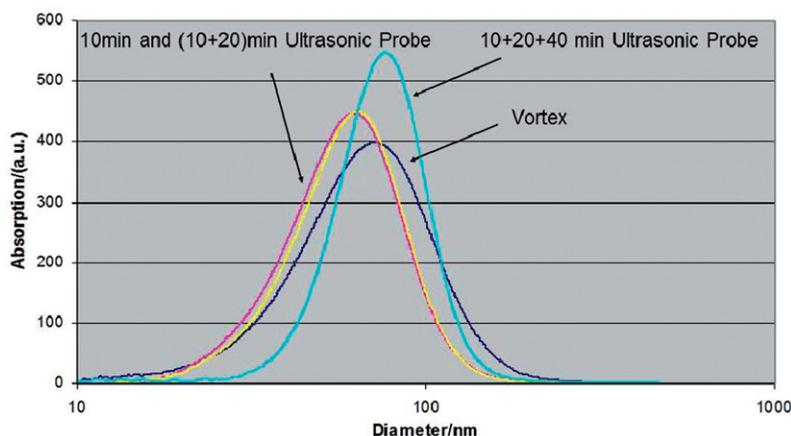
Figure 4. CPS analysis of a CeO<sub>2</sub> sample re-dissolved using simple vortexing (blue line) or a combination of vortexing and ultrasonic treatment for 10 s (yellow line), 30 s (pink line) and 70 s (cyan line).
