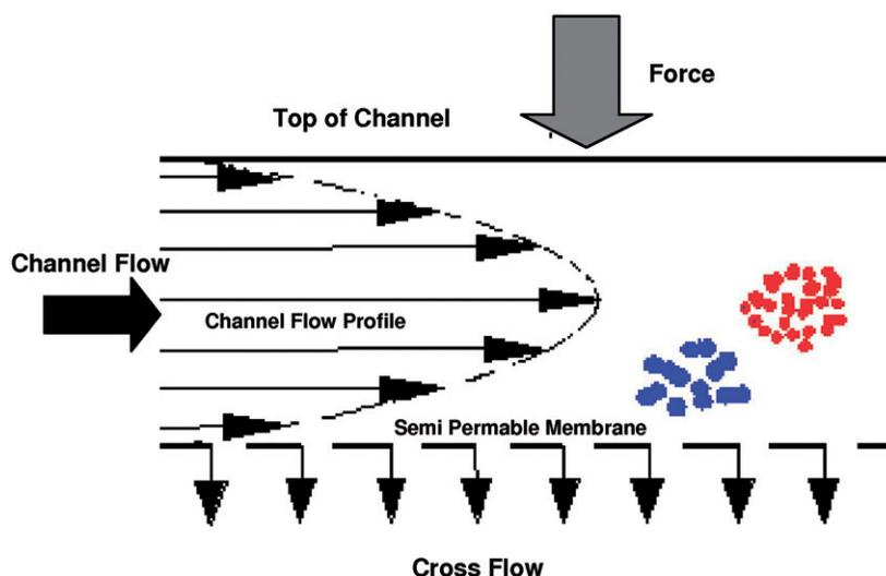
Figure 2. Schematic view of a flow field flow separation channel showing smaller particles moving closer to the centre of the channel in a higher velocity zone and thus existing before larger particles.
