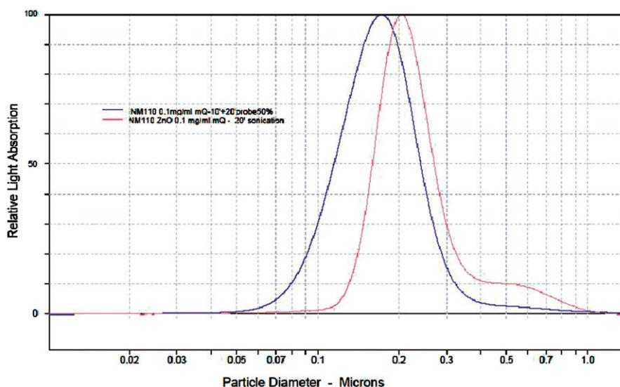
Figure 3. Size distribution obtained by CPS analysis of a ZnO sample dissolved in water and treated with ultrasonic probe for varying time periods of 20 s (right curve) or 30 s (left curve).
