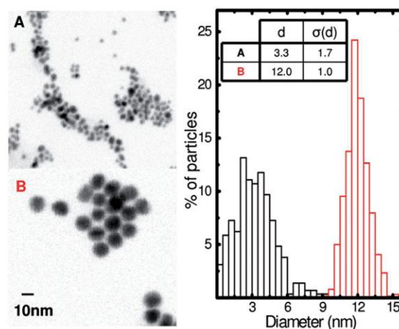
Figure 1. Scanning electron microscopy (SEM) analysis of two samples of citrate-stabilised gold nanoparticles of different sizes: (A) SEM micrograph of 3 nm gold nanoparticles; (B) SEM micrograph of 12 nm gold nanoparticles; and (C) particle size distribution obtained by semiautomatic image analysis of sample A (left) and B (right).
