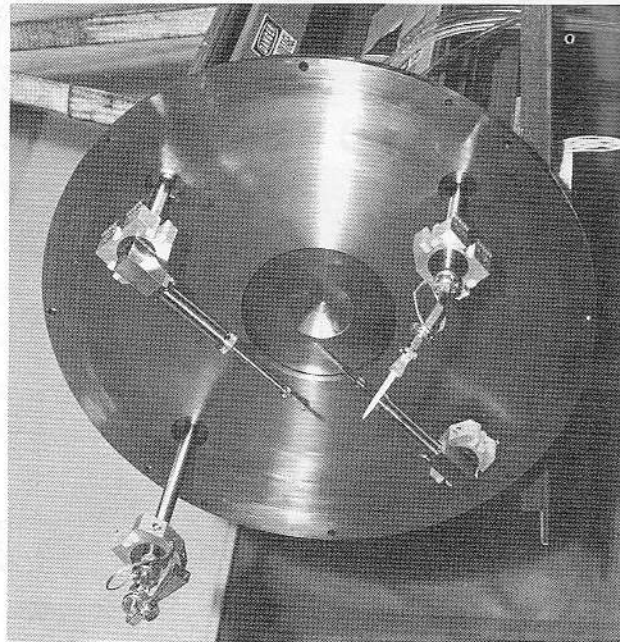
FIG. 9.47 Probe and waveguide assemblies mounted in tubing introduced through a vacuum wall with Wilson seals. The probe carts move on rails inside the vacuum system, allowing accurate positioning. (Courtesy of General Atomic, San Diego, Calif.)
