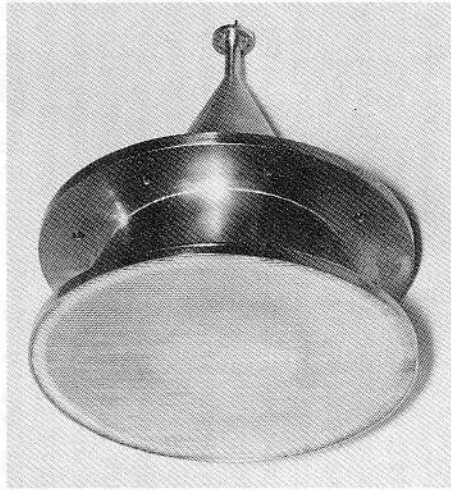
FIG. 9.27 Dielectric microwave lens, using impedance matching grooves. (Courtesy TRG, Inc.)
