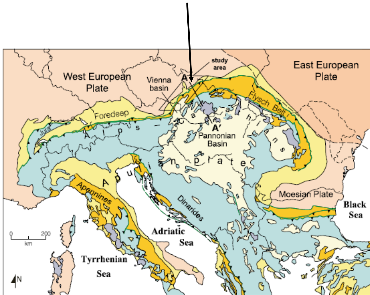
Figure 1. Generalized geologic map of the Alpine–Carpathian orogenic system of Europe. Study area is located in the box. The inner zones of the Alpine–Carpathian orogen are shown in blue. Modified from Picha (1996). Cross section of AA' is shown in Figure 2. Golonka et Picha (2006)
