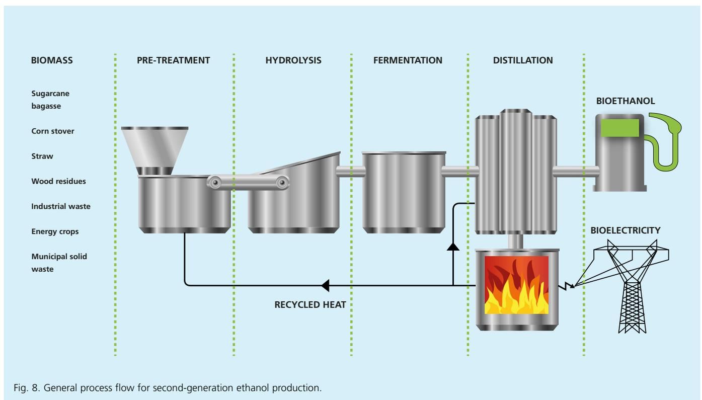
Fig. 8. General process flow for second-generation ethanol production.
