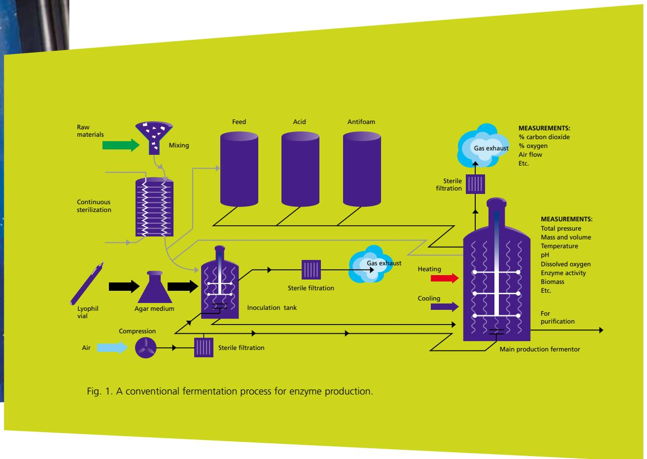
Fig. 1. A conventional fermentation process for enzyme production.
