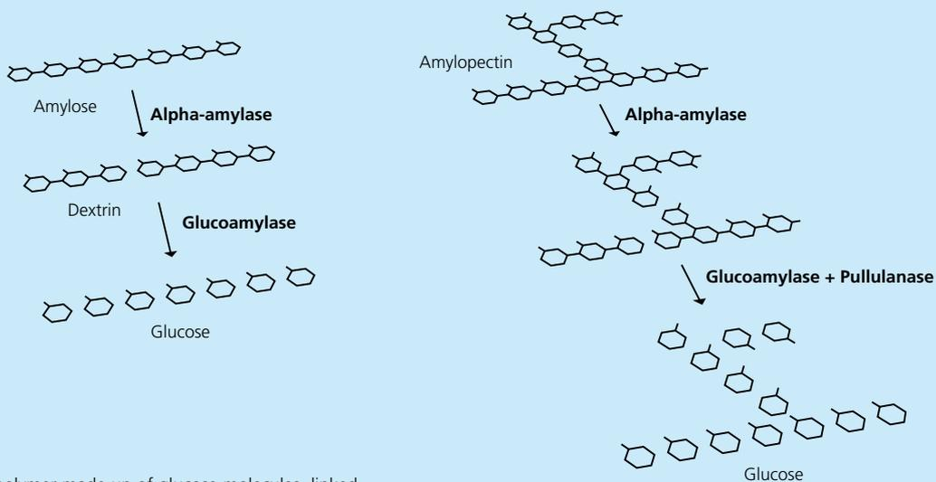
Native starch is a polymer made up of glucose molecules linked together to form either a linear polymer called amylose or a branched polymer called amylopectin. Glucose units are linked in a linear way with alpha-1,4-glycosidic bonds. The branching in amylopectin takes place with alpha-1,6-glycosidic bonds occurring at every 24-30 glucose molecules.
