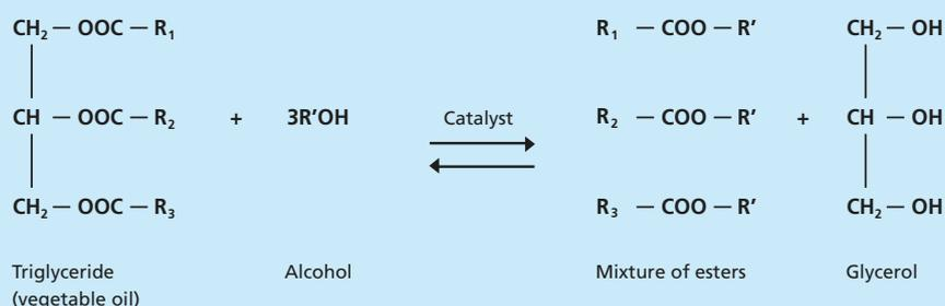
Fig. 9. Transesterification reaction of triglycerides.
