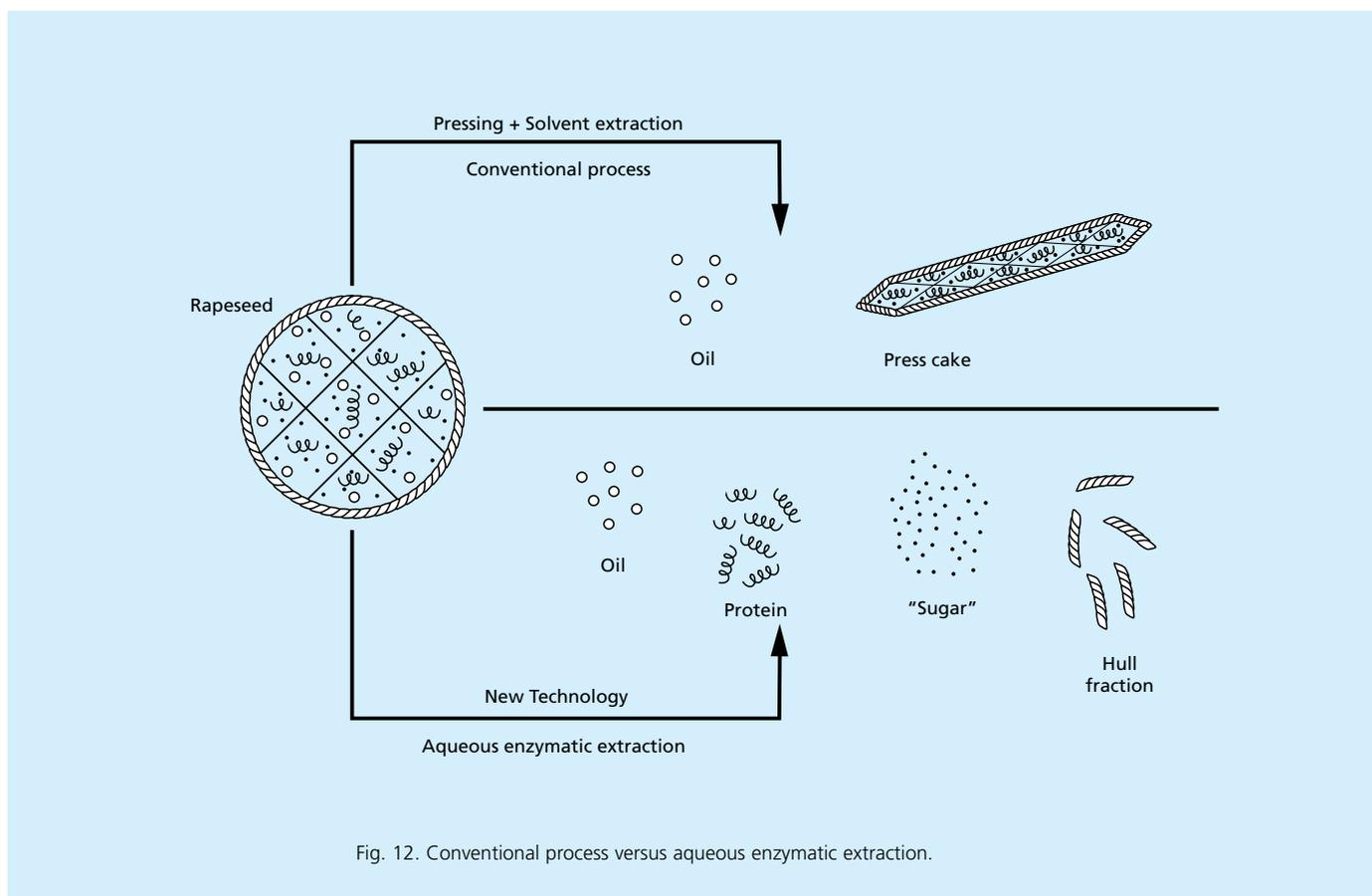
Fig. 12. Conventional process versus aqueous enzymatic extraction.
