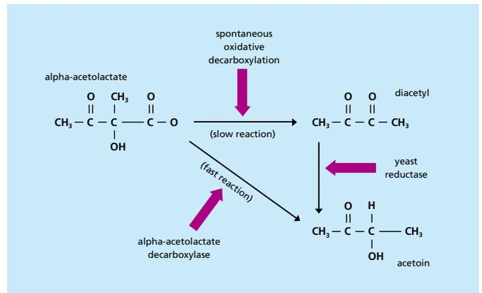
Fig. 22. The removal of alpha-acetolactate during fermentation.
