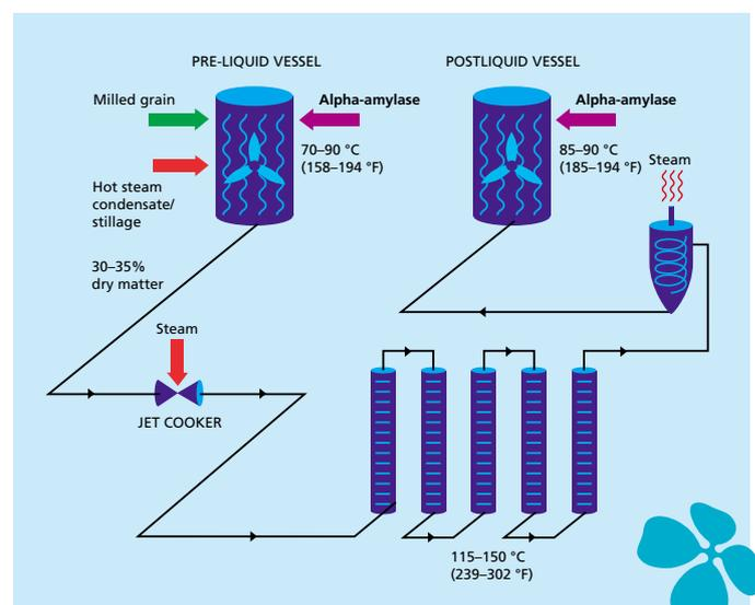
Fig. 5. Warm or hot slurry liquefaction processes.
