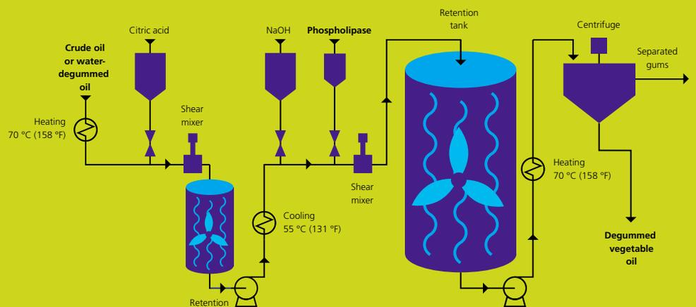
Fig. 26. Degumming of lipid oil with phospholipase.
