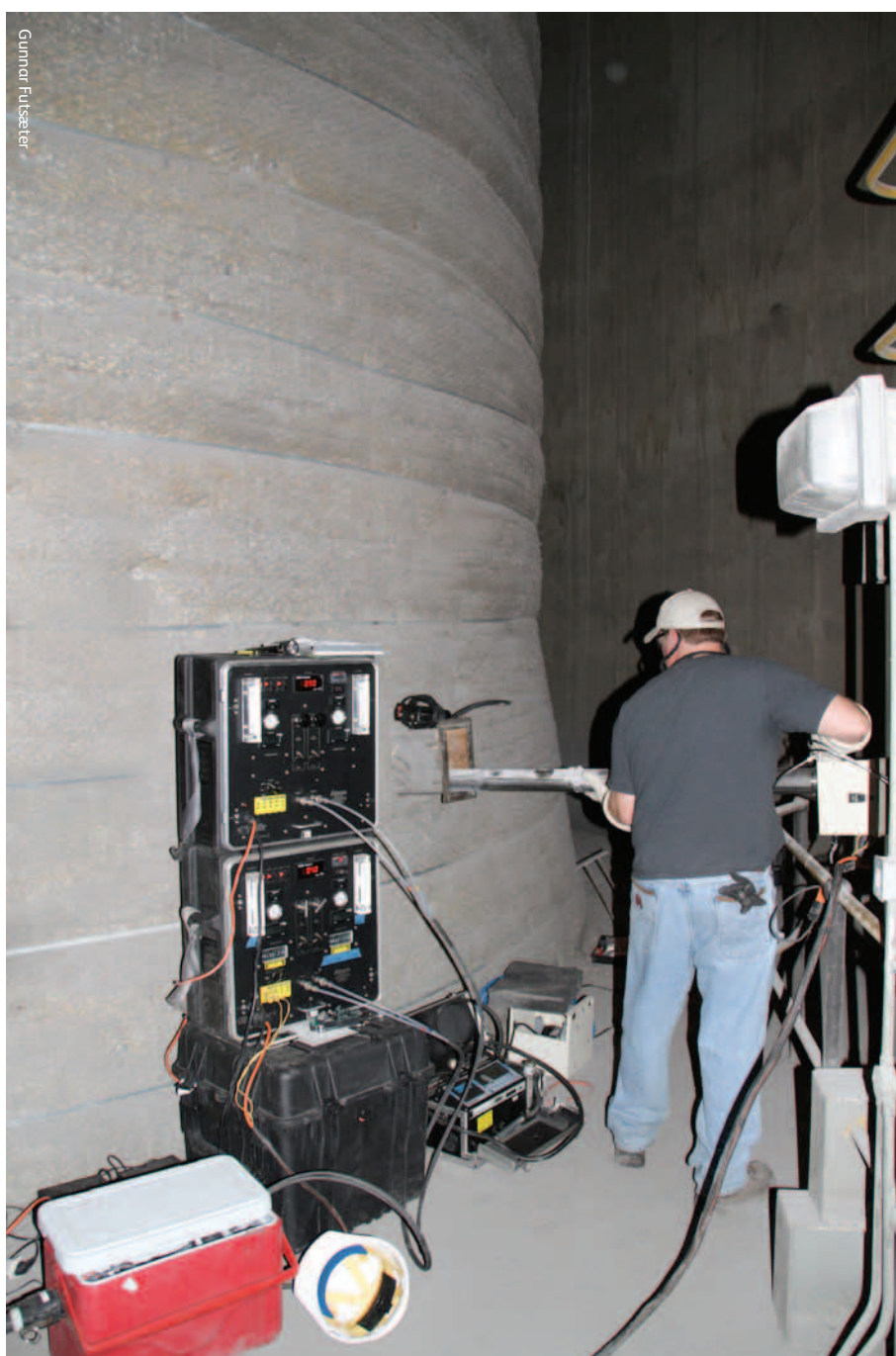
Sampling of mercury emissions at the Kendal coal-fired power plant in South Africa, conducted under a UNEP project. A probe with mercury traps is inserted into a sampling port in the stack to collect mercury present in the flue gas. The mercury traps are subsequently analysed according to the US EPA Mercury Monitoring Toolkit sampling protocol.
