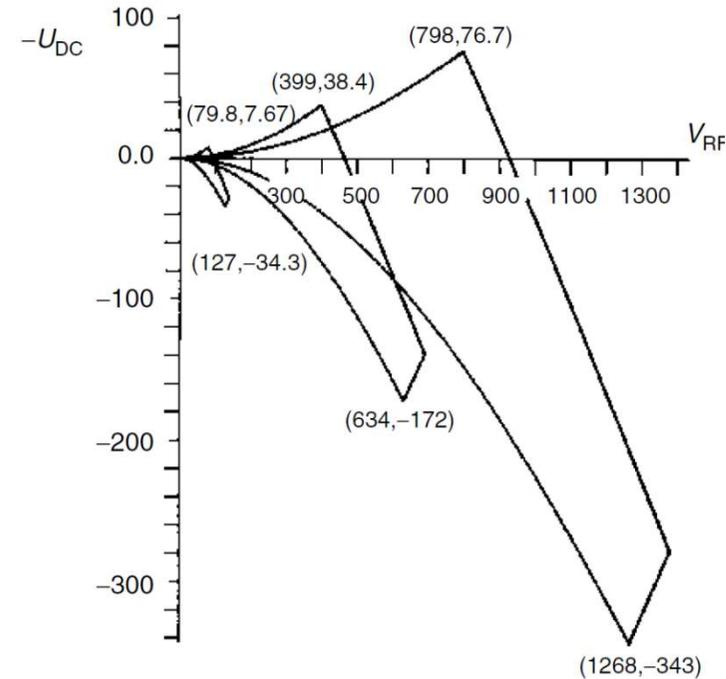
Typical stability diagram for a 3D ion trap. The value at  $\beta_z = 1$  along the  $q_z$  axis is  $q_z = 0.908$ . At the upper apex,  $a_z = 0.149\ 998$  and  $q_z = 0.780\ 909$ .
