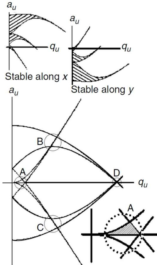
Stability areas for an ion along  $x$  or  $y$  and along  $x$  and  $y$ ;  $u$  represents either  $x$  or  $y$ . The four stability areas are labelled A to D and are circled.
