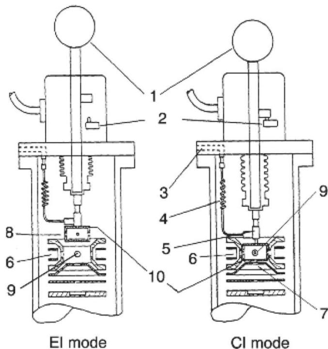
Chemical ionization consists of producing ions through a collision of the molecule to be analysed with primary ions present in the source (with ions of a **reagent gas** that are present in the ion source). Ion–molecule collisions will thus be induced in a definite part of the source. In order to do so, the local pressure has to be sufficient to allow for frequent collisions.
