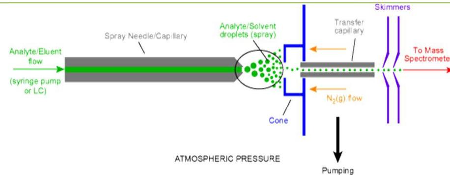
ESI is produced by applying a strong electric field, under atmospheric pressure, to a liquid passing through a capillary tube with a weak flux (normally  $1\text{--}10\ \mu\text{Lmin}^{-1}$ ). The electric field is obtained by applying a potential difference of 3–6 kV between this capillary and the counter-electrode, separated by 0.3–2 cm, producing electric fields of the order of  $10^6\ \text{Vm}^{-1}$
