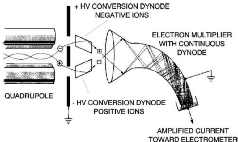
A type of **continuous-dynode** electron multipliers (CDEM), which is called a **channeltron**, is made from a lead-doped glass with a curved tube shape that has good secondary emission properties.
