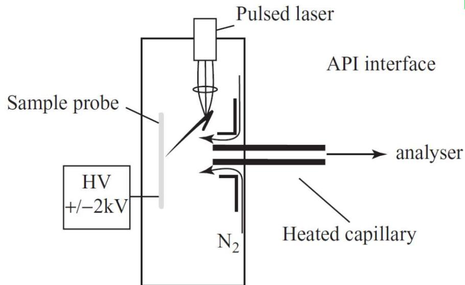
As the transfer of ions into the mass spectrometer is **relatively inefficient**, the total sample consumption is higher for AP-MALDI than for vacuum MALDI.
