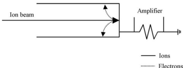
Because the charge associated with an electron leaving the wall of the detector is identical to the arrival of a positive ion at this detector, **secondary electrons** that are emitted when an ion strikes the wall of the detector are an important source of errors if they are not suppressed. The accuracy of this detector can be improved by preventing the escape of reflected ions and ejected secondary electrons.
