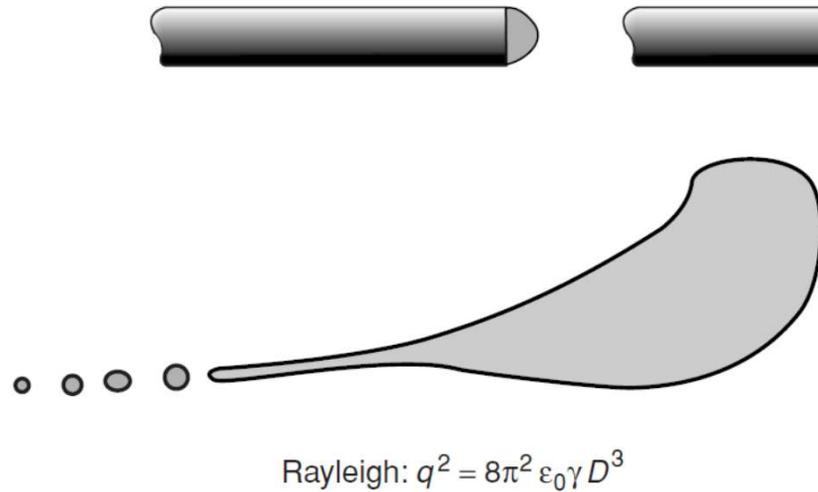
A decomposing droplet in an electrospray source;  $q$ , charge;  $\epsilon_0$ , permittivity of the environment;  $\gamma$ , surface tension and  $D$ , diameter of a supposed spherical droplet.
