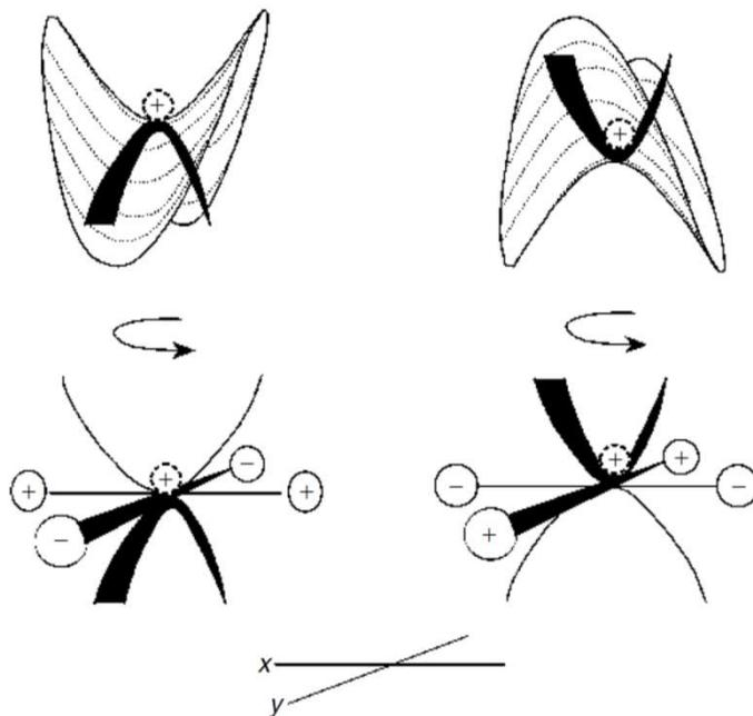
It goes down the potential ‘valley’ with respect to the negative rods, and acquires some kinetic energy in that direction. However, the potentials quickly change, so that the **kinetic energy** is converted into **potential energy** and the ion goes back to the centre of the rods, as would happen for a ball on a horse’s saddle that is turned quickly. The name ‘**saddle field**’ is an allusion to this phenomenon.
