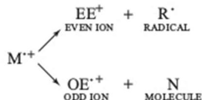
These two types of ions have different chemical properties. Each primary product ion derived from the molecular ion can, in turn, undergo fragmentation, and so on. All these ions are separated in the mass spectrometer according to their mass-to-charge ratio,
