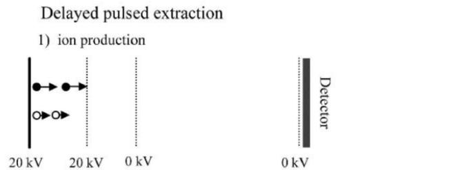
So, delayed pulsed extraction corrects the energy dispersion of the ions leaving the source with the same  $m/z$  ratio and thus improves the resolution of the TOF analyzer.
