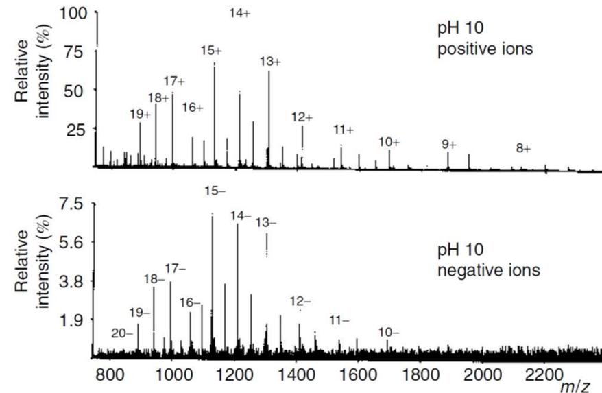
Charges of ions generated by ESI do not reflect the charge state of compounds in the analysed solution, but are the result of both **charge accumulation** in the droplets and **charge modification** by electrochemical process at the probe tip.
