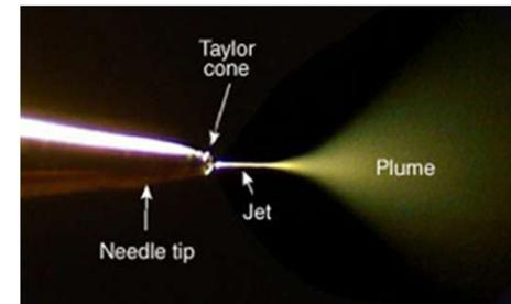
*Breakdown of the droplets can occur before the limit given by the **Rayleigh equation** is reached because the droplets are mechanically deformed, thus reducing the repulsion necessary to break down the droplets. The solvent contained in the droplets evaporates, which causes them to shrink and their charge per unit volume to increase.*
