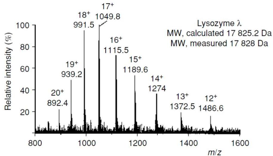
ESI spectrum of phage lambda lysozyme. The molecular mass is measured as being  $17\,828 \pm 2.0$  Da.
