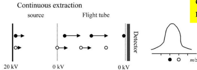
The extraction pulse applied after a certain delay transmits more energy to the ions which remained for a longer time in the source. Consequently, the initially less energetic ions receive more kinetic energy and join the initially more energetic ions at the detector.
