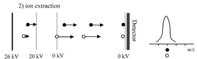
Lower pulse voltages or shorter delays are required to focus ions of lower  $m/z$  ratio. In general, for a given  $m/z$  and initial velocity distribution, greater voltage pulses require shorter time delays and vice versa.
