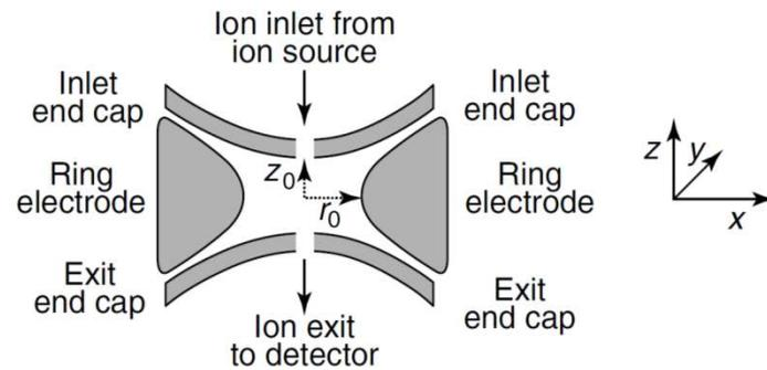
In the Paul ion trap the motion of the ions under the influence of the applied potentials occurs in three dimensions,  $x$ ,  $y$  and  $z$ . The  $z$  motion resulting from the kinetic energy of the ions when they enter the quadrupole field. However, due to the cylindrical symmetry  $x^2 + y^2 = r^2$ , it can also be expressed using  $z$ ,  $r$  coordinates.
