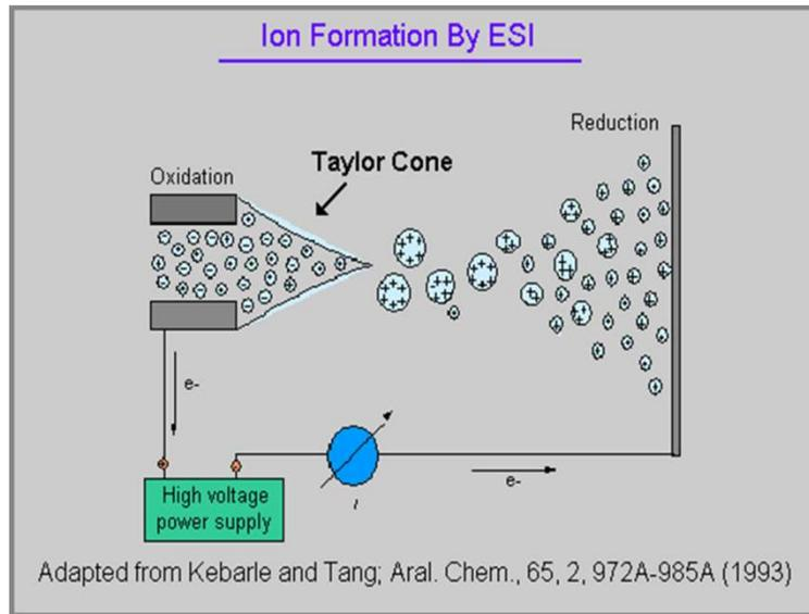
When positive ions are extracted for analysis, electrons have to be provided in the circuit from the capillary. The same number of negative charges must be 'pumped' out of the solution as positive charges are extracted to the analyser, thus an **oxidation** occurs. For negative ions, electrons have to be consumed, and thus a **reduction** occurs.
