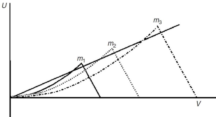
Stability areas as a function of  $U$  and  $V$  for ions with different masses ( $m_1 < m_2 < m_3$ ). Changing  $U$  linearly as a function of  $V$ , we obtain a straight operating line that allows us to observe those ions successively.
