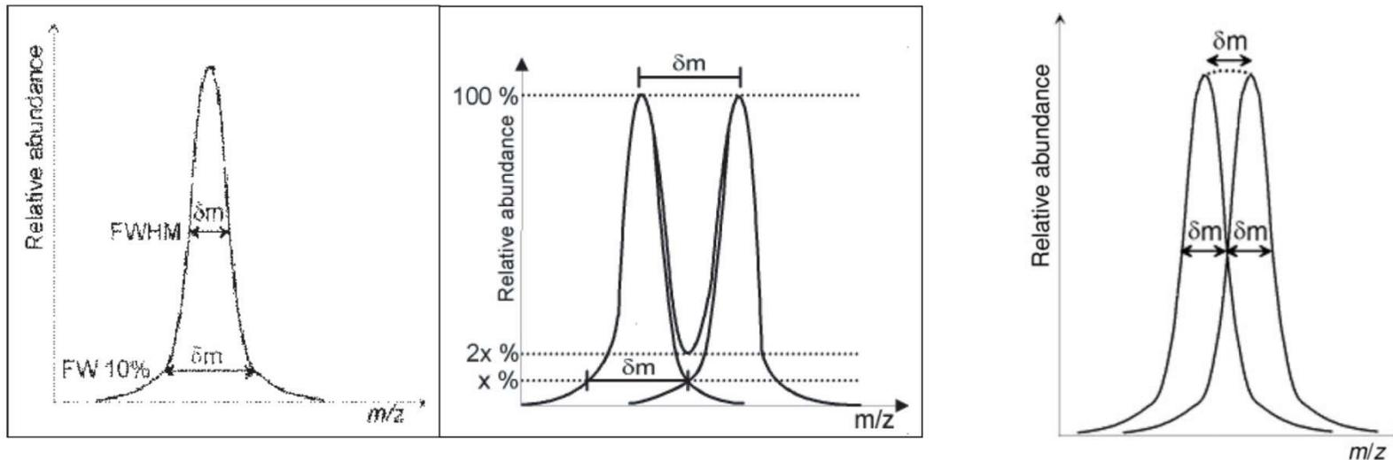
Relationship between the two definitions of resolution, resolution full width at  $x\%$  of the peak height or resolution at  $y\%$  of the valley. As the bottom of the valley is the sum of the intensities at the cross,  $y = 2x$ .
