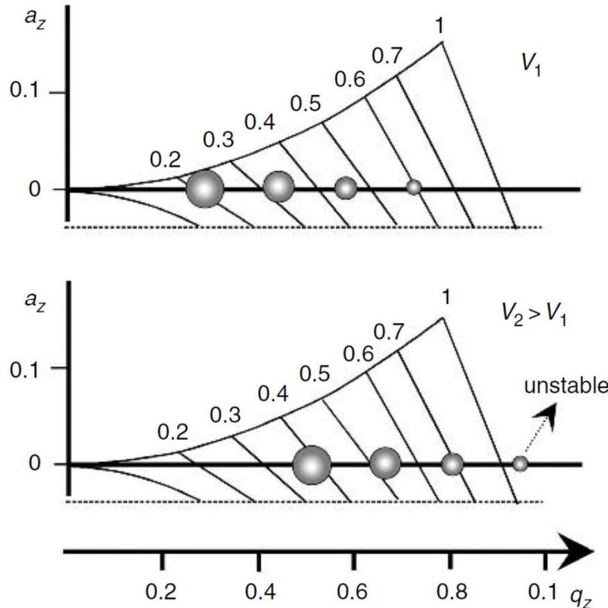
If  $V$  is increased, all the ions will have a higher  $q_z$  value. If this value is equal to **0.908**,  $\beta = 1$ , and the ion has reached its stability limit. A slight increase of  $V$  will cause this ion to have an unstable trajectory, and will be expelled from the trap in the  $z$  direction.
