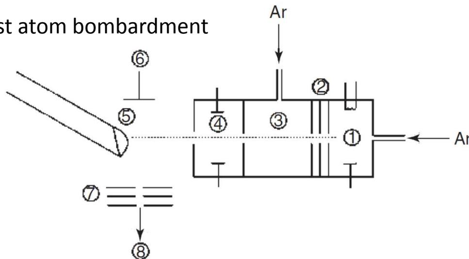
Softer than EI and CI. Ions are produced by bombardment with heavy atoms. Gives  $(M+H)^+$  ions and little fragmentation. Good for more polar compounds.
