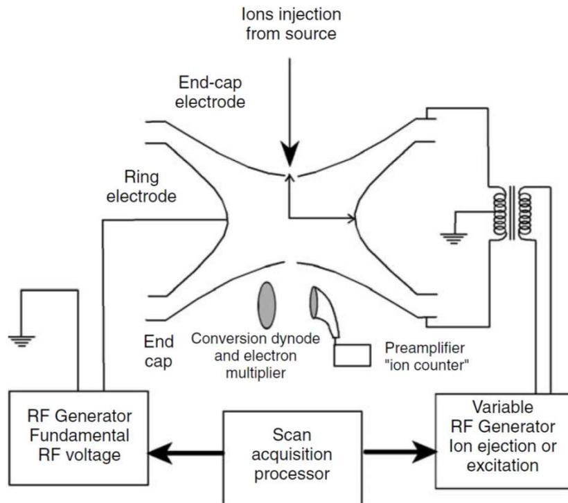
Ion trap with an RF voltage applied to the ring electrode, providing the fundamental frequency  $\nu$  and its associated variable amplitude  $V$ . Instead of injecting ions, electrons may be injected for internal ionization. Variable RF voltage can be applied to the end caps for ion excitation or ion ejection.
