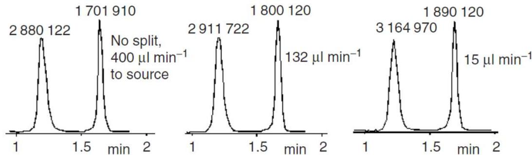
Another feature of ESI is its sensitivity to concentration, and not to the total quantity of sample injected in the source, as is the case for most other sources.
