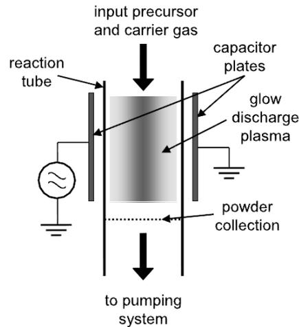
Fig. 10 General layout of a capacitive-coupled RF system for nanoparticle synthesis working at reduced pressure.
