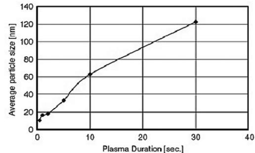
Fig. 12 Average particle size, obtained in a device according to Fig. 11, as a function of the plasma duration, which is the dwell time of the particles in the plasma.<sup>20</sup> Reproduced by permission of Springer.
