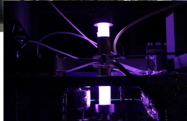
Low pressure surface-wave microwave discharge 2,45 GHz,
