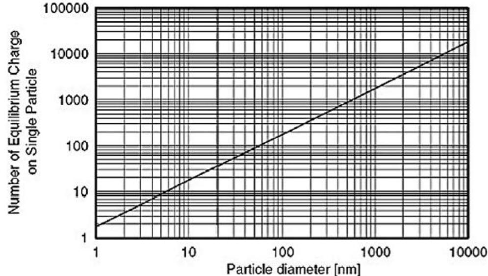
Fig. 9 Average number of electric charges carried by a single nanoparticle. The particle charge increases linearly with the diameter over many orders of magnitude.<sup>20</sup> Reproduced by permission of Springer.
