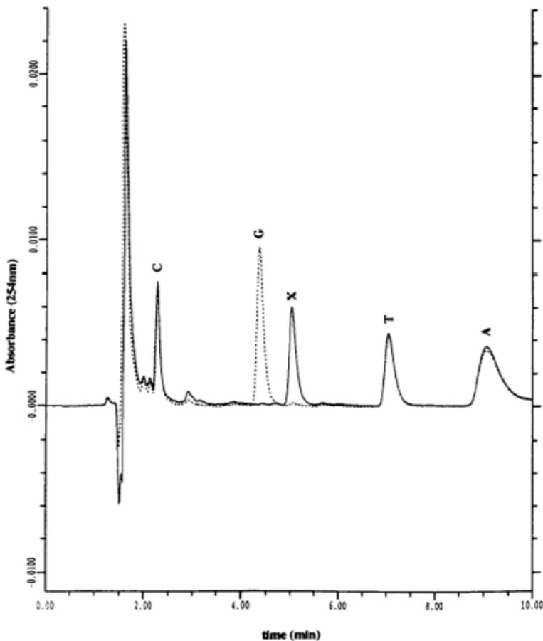
Fig. 4. Effect of guanase on bases derived from a formic acid hydrolysate of calf thymus DNA. Samples were HPLC with UV detection prior to (---) and following (—) guanase treatment as described in Materials and Methods. G, guanine; X, xanthine; T, thymine; A, adenine.
