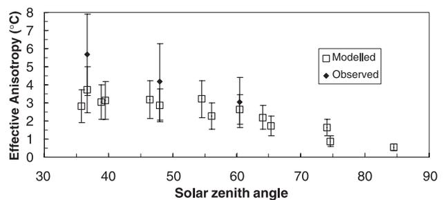
Fig. 6. Observed and modelled thermal anisotropy for a 45° off-nadir sensor (12° FOV) at 650 m during one summer day (YD 228 1992) over a simple urban surface (Table 2). Error bars represent ± 1 standard deviation.
