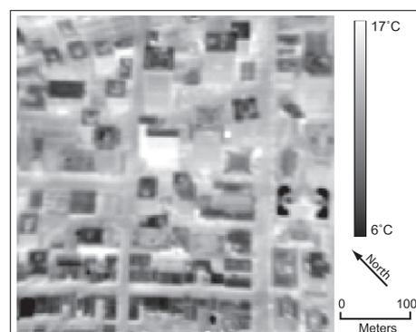
Fig. 4. Thermal image of downtown Vancouver, obtained from an airborne thermal scanner illustrating nighttime temperature variations from a small off-nadir viewing angle. Rooftops are cool relative to building walls and streets. The image is corrected for atmospheric effects.
