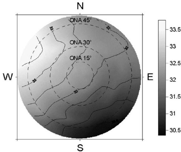
Fig. 5. Modelled directional brightness temperatures for an airborne thermal scanner (12° FOV) viewing a simple urban surface (Table 2) from an elevation of 650 m for a mid-morning simulation (YD 228, 1992) using S3mod (Soux et al., 2000). The image plots sensor-detected brightness temperature interpolated from modelled values at 5° azimuthal and off-nadir steps.
