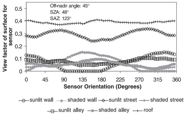
Fig. 3. View factors of urban surface components for an airborne thermal scanner sensor calculated using the S3mod model (Soux et al., 2000) for the light industrial area of Vancouver BC (Table 2). YD 228 1992, 1030 LDT.
