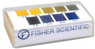
Suitable range indicator papers (pH 5.0 – 9.0) are used for approximate pH measurements, for instance to detect the acidification of an organism
