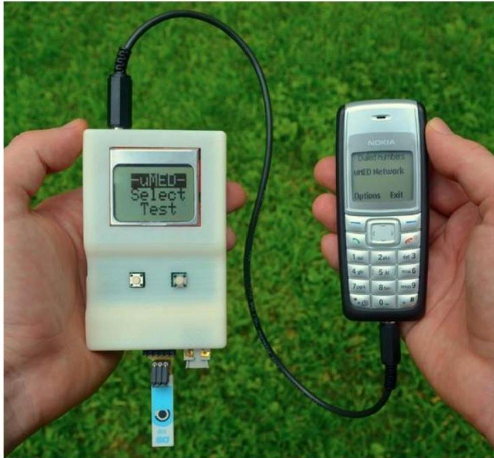
A universal mobile electrochemical detector (uMED). The uMED device (left) can perform a variety of electrochemical analyses on commercial and custom electrodes. Results can be transferred through the audio jack of any phone to enable connectivity (right).
