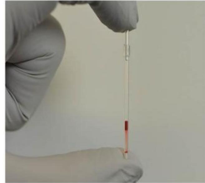
A low-cost, rapid test for sickle cell disease. After centrifugation over an aqueous multiphase system, blood cells from a donor with sickle cell disease separate by density. Dense cells characteristic of sickle cell disease form a red layer at the bottom of the test.
