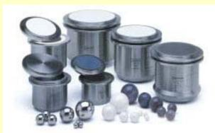
Particles repeatedly subjected to deformation, cold welding, and fracture, homogenization on an atomic scale
