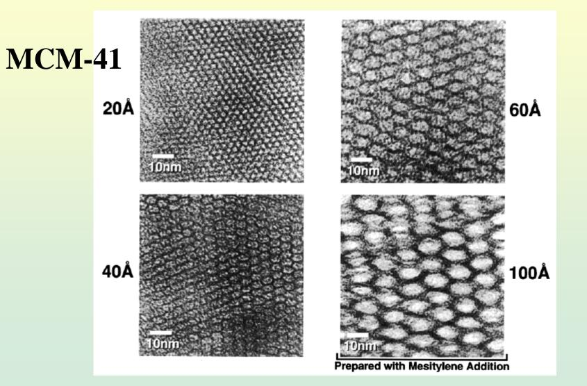
**Surfactant chain length - increasing the chain length = bigger pores**
