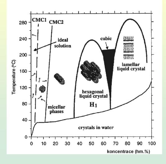
Phase diagram of  $C_{16}$ TMABr CMC = critical micelle conc.
