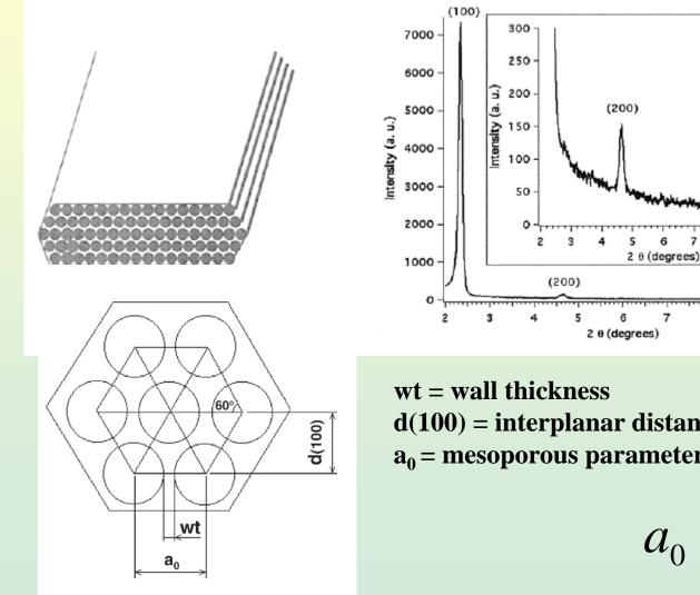
d(100) = interplanar distance in the (100) plane **a**<sub>0</sub> = mesoporous parameter
