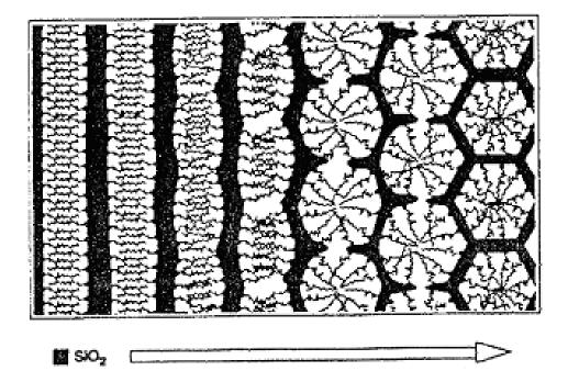
As condensation proceeds the charge on the silicate layer decreases
