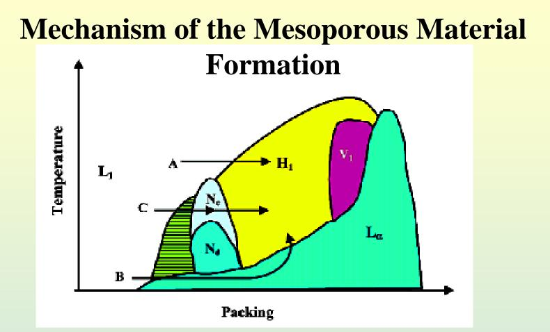
$L_1$ = micellar solution; Nc = nematic phase;  $H_1$  = normal hexagonal phase (MCM-41; SBA-15);  $V_1$  = normal bicontinuous cubic phase (MCM-48);  $L_{\alpha}$  = lamellar phase (MCM-50)
