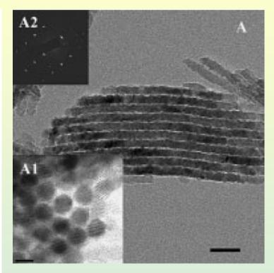
Cr<sub>2</sub>O<sub>3</sub> crystalline nanowires (bar = 25 nm for A, 10 nm for A1)
