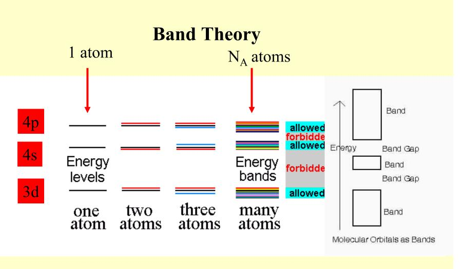
Energies of electrons are quantized = can possess only allowed energies, can occupy only allowed levels, cannot enter forbidden band gaps.
