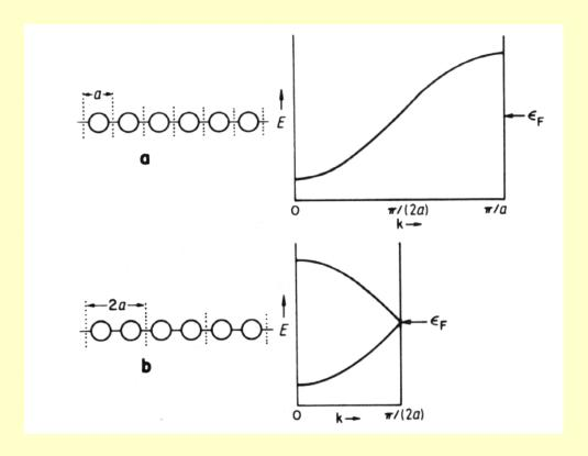
Peierls distortion – maximizing bonding, lowering the DOS at the Fermi level, bonding states down in energy, antibonding states up, a band gap opens at the Fermi level
