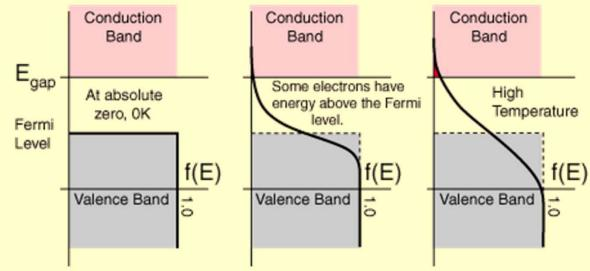
No electrons can be above the valence band at 0K, since none have energy above the Fermi level and there are no available energy states in the band gap.
