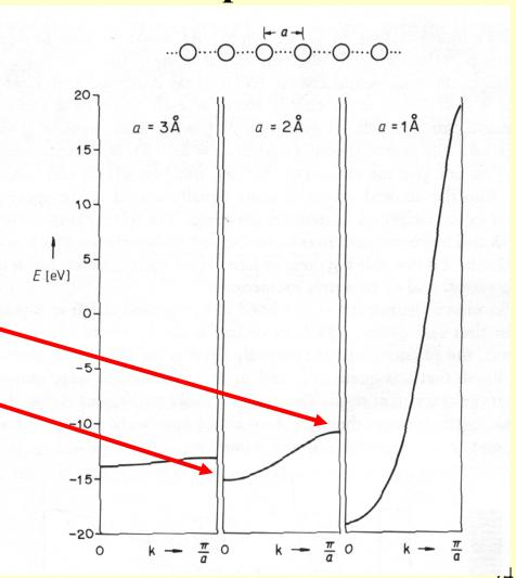
Different types of orbitals (symmetry) form separate bands s, p, d bands
