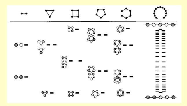
A rough rule of thumb: the separation of the energy levels in the dimer corresponds to about half width of the energy band.
