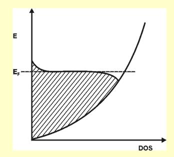
The Fermi level cuts a band in a metal
