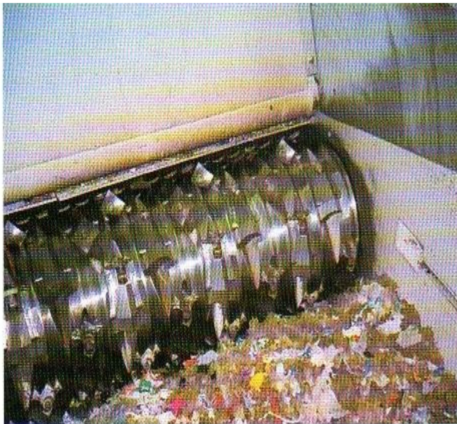
Mixed plastic input is preshredded to reduce it to particle sizes of 10 to 40 mm.
