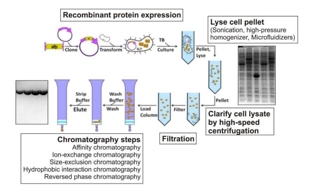
**Figure 3.** Workflow of recombinant protein purification includes (i) the lysis of a cell pellet by sonication or high-pressure homogenizer, (i) the clarification of cell lysate by high-speed centrifugation, (iii) filtration, and (iv) one or more chromatographic purification steps.
